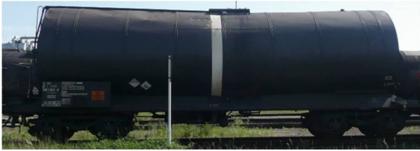
Fig. 1 Tank wagon for the transport of liquid petrochemical products [14]
