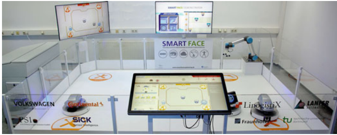
Fig. 9 Initial prototype of production planning and control concepts presented at the Hanover Fair 2015. Within the SMART FACE project a simple, miniaturized and very abstract model of an industrial cyber-physical production system has been implemented. Two miniaturized AGVs representing the assembly order (car models) and two AGVs showing the parts supply (visualized by tablets showing the delivered parts)
