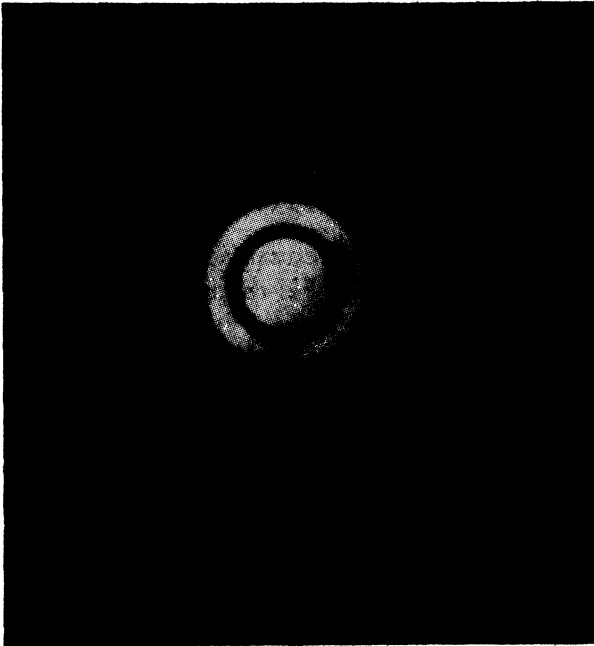
FIG. 15. Centric (diffraction figure at the center of curvature of a spherical wave which has passed through a diaphragm with a circular rim; sometimes called “Airy spurious disk”)
