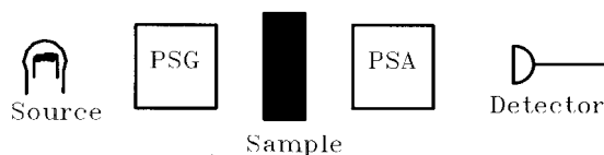
FIGURE 1 A sample-measuring polarimeter consists of a source, polarization state generator (PSG), the sample, a polarization state analyzer (PSA), and the detector. (After Chenault, 1992.)
