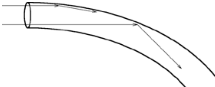
FIGURE 7 X-rays traveling in a bent capillary tube. The ray entering at the bottom (closest to the center of curvature) strikes at a large angle. (Adapted from Ref. 15.)
