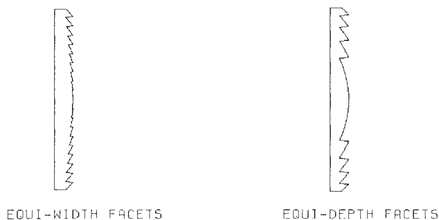
FIGURE 6 Two main types of Fresnel lenses: equi-width and equi-depth.
