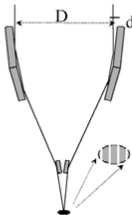
FIGURE 9 Schematic drawing of a grazing-incidence X-ray interferometer.
