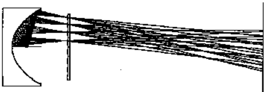
FIGURE 45 Reflector with array of concave facets and an array of lenslets. The lenslets image the facets.
