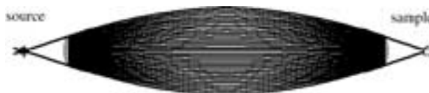
FIGURE 10 Sketch of the interior channels of a monolithic polycapillary optic. Monolithic optics can be focusing, as shown, or collimating, as in Fig. 9. (Sketch from Ref. 12.)
