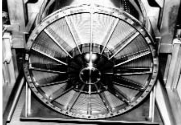
FIGURE 2 An X-ray optics module for the XMM observatory. Fifty-eight electroformed nickel Wolter-I optics are nested to increase the effective X-ray collecting area. ( Photo courtesy of ESA. )
