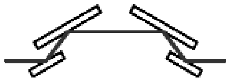
FIGURE 4 Two monolithic double reflectors arranged in a high-resolution configuration.
