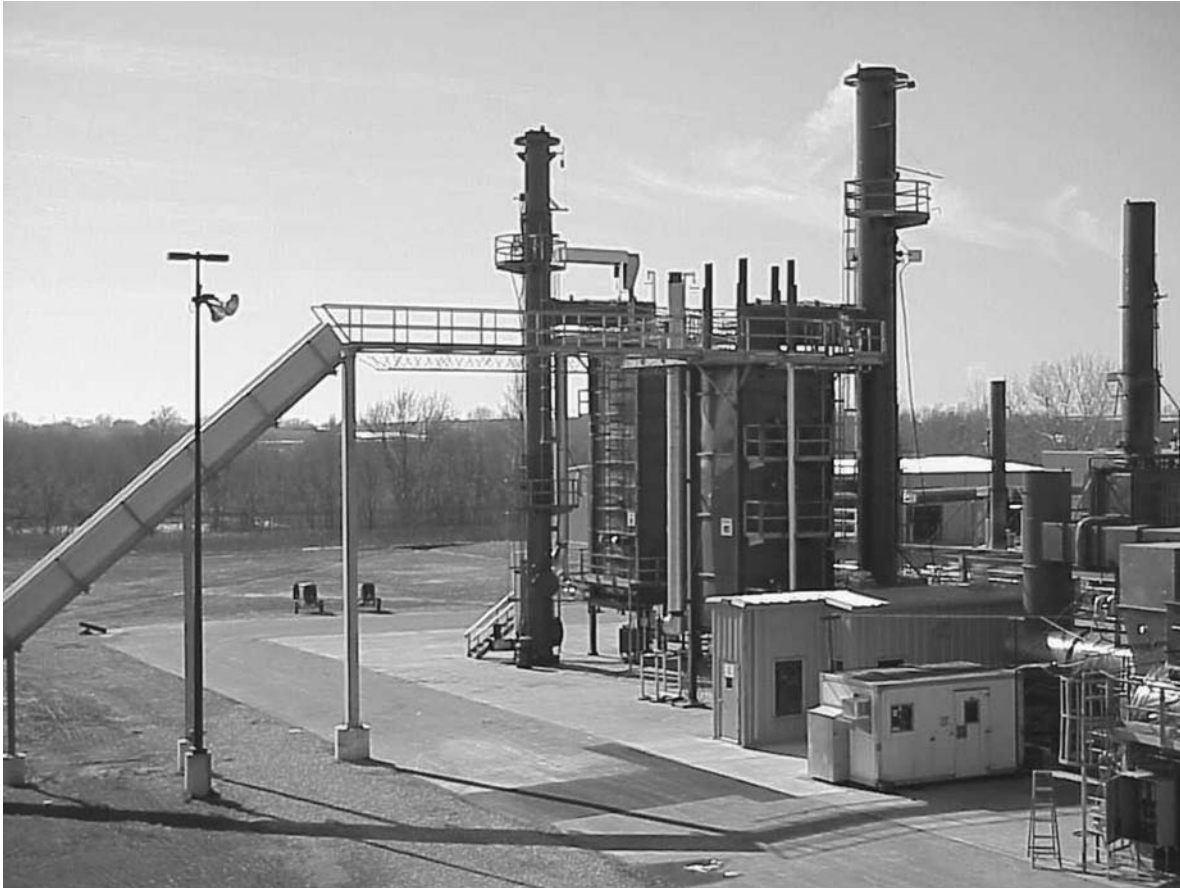
FIGURE 9.3 Test furnace for simulation of downfired tests. (Courtesy of John Zink Co., LLC. 21 )
