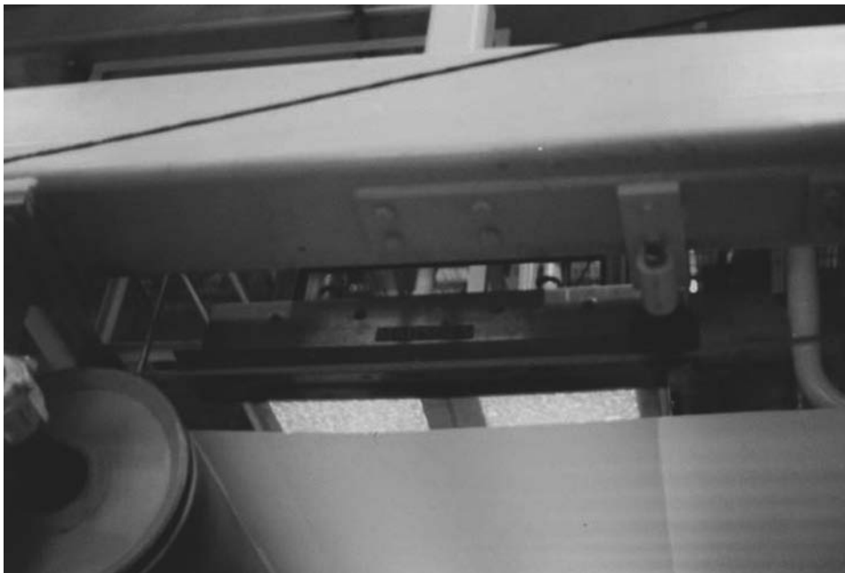
FIGURE 13.15 Infrared burner heating a continuously moving paper web. (Courtesy of Marsden, Inc. 19 )
