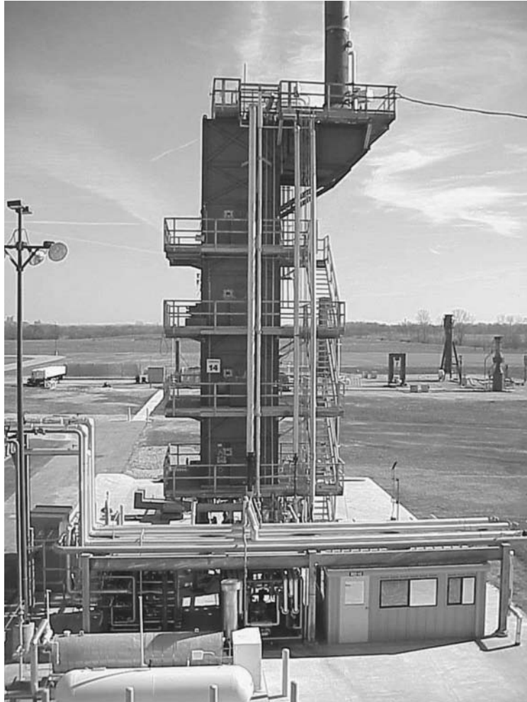
FIGURE 9.2 Test furnace for simulation of ethylene furnaces. (Courtesy of John Zink Co., LLC. 21 )
