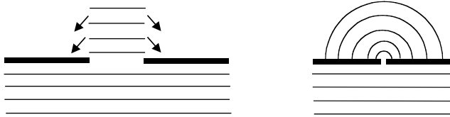
FIGURE 7.14 Large aperture has a very little effect on the plane wavefront that passes through it. Small aperture will turn the plane wavefront that penetrates the hole into a hemispherical wavefront because of the closeness of the new point sources.
