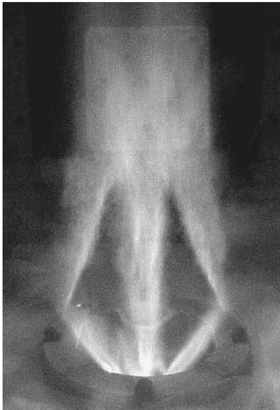
FIGURE 6.2 Example of a low-luminosity gas flame. (Courtesy of John Zink Company, LLC. 3 )
