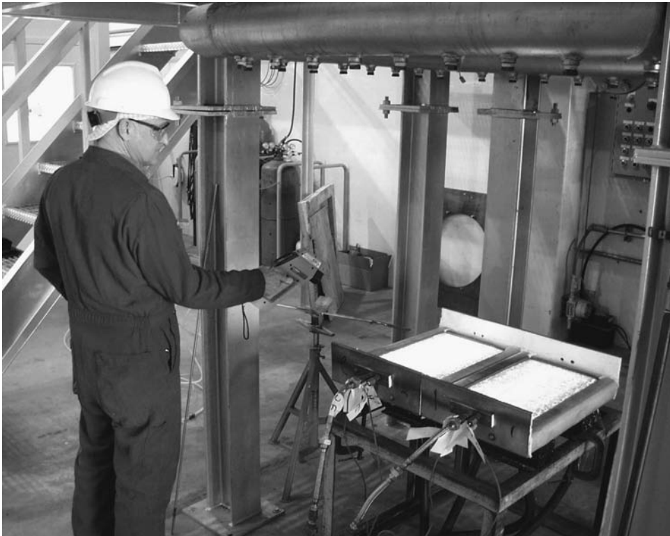
FIGURE 13.31 Example of an infrared pyrometer measuring the surface temperature of a porous refractory matrix burner. 19
