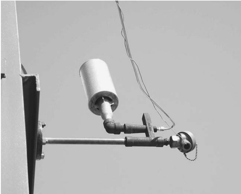
FIGURE 9.8 Suction pyrometer with noise muffler.
