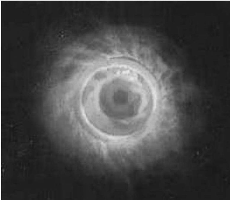
FIGURE 17.14 Ultra-low-NO x burner flame.
