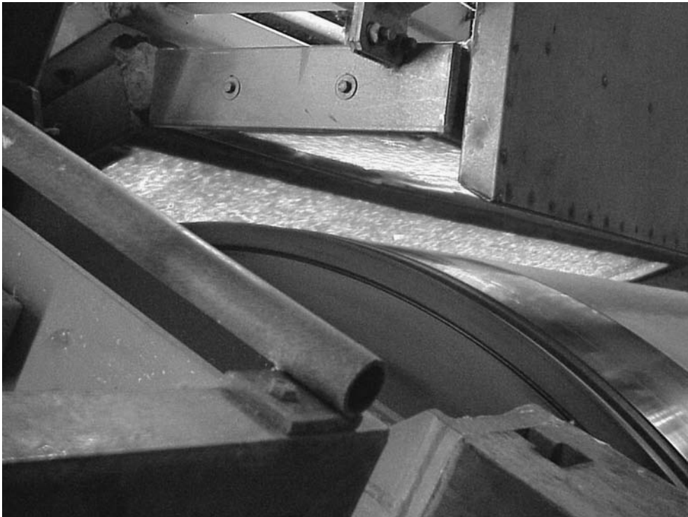
FIGURE 13.17 Supplemental IR burners for paper drying located over steam cylinders. (Courtesy of Marsden, Inc.)
