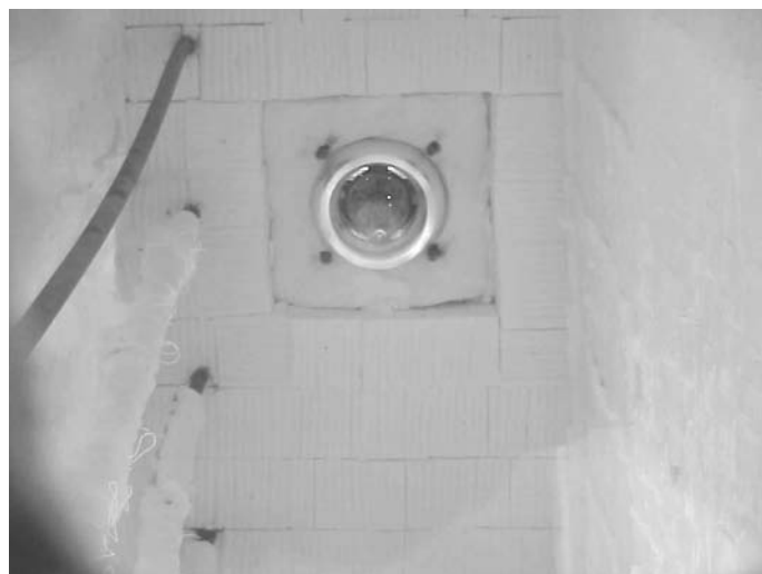
FIGURE 16.4 Down-fired burner commonly used in top-fired reformers. (Courtesy of John Zink Co., LLC. 3 )
