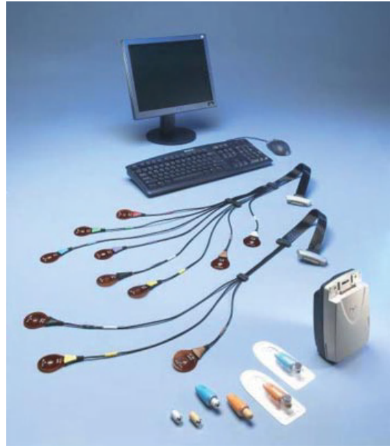
Figure 5.9 The capsule imaging system comprising the capsule endoscope, a data recording device, and a computer workstation.
