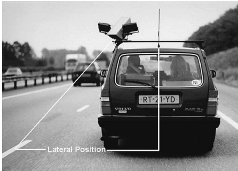
Figure 30.1. The instrumented car. Note that the camera for lateral position measurements is equipped with two infrared lights, to enable recording during the night and dark weather circumstances.
