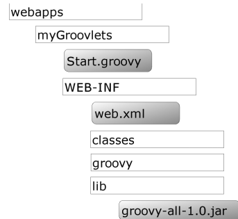
Figure 9.6 Directory structure for a sample Groovlet web application below the webapps dir
