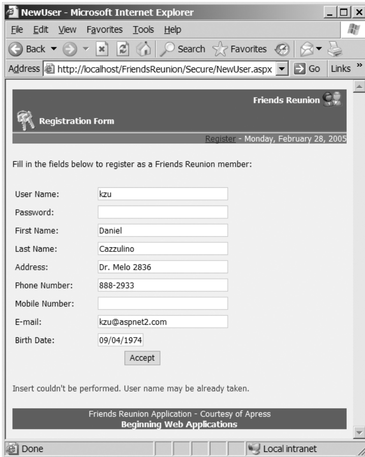
Figure 4-3. An error message appears when you try to add a user whose name already exists in the database.
