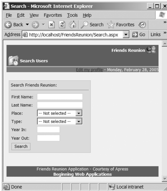
Figure 6-5. On the Search page, selective controls' visibility depends on the session state items.
