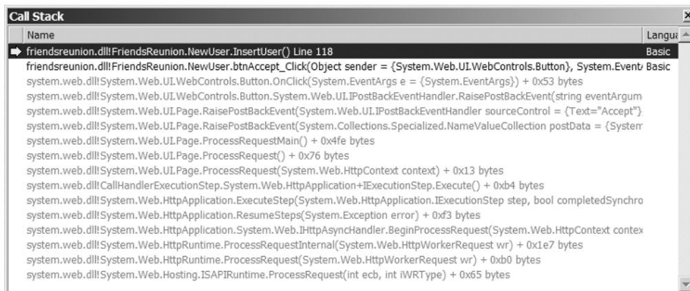
Figure 11-24. When the Show Non-user Code option is selected, the Call Stack window shows the entire code path.
