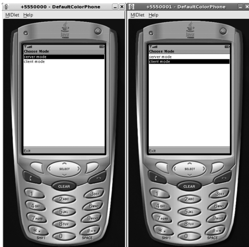
Figure 7-1. When the Bluetooth Checkers game begins, one player chooses to act as the server and the other chooses to act as the client.
