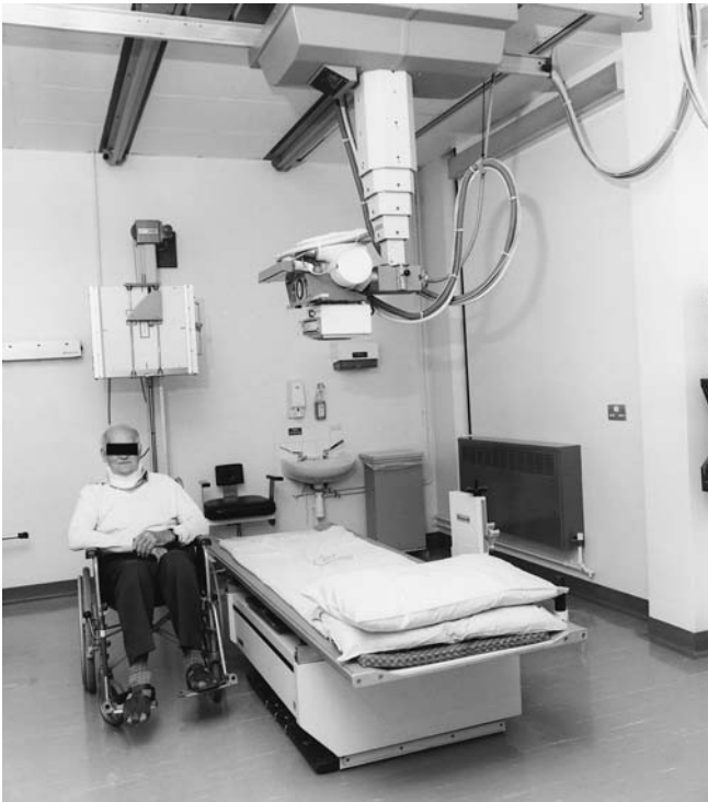
Figure 2 Elevating adjustable height, floating table top X-ray examination table
