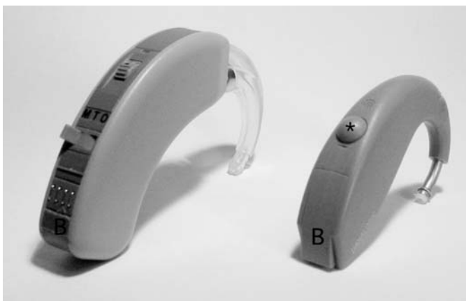
Figure 5 Modern, behind the Ear (BTE) hearing aids. On the left is one with conventional patient controls including a volume control wheel. On the right is a digital aid that can be programmed to a number of different settings. The button marked with an asterisk is used to cycle through the different programs. B indicates the battery compartments
