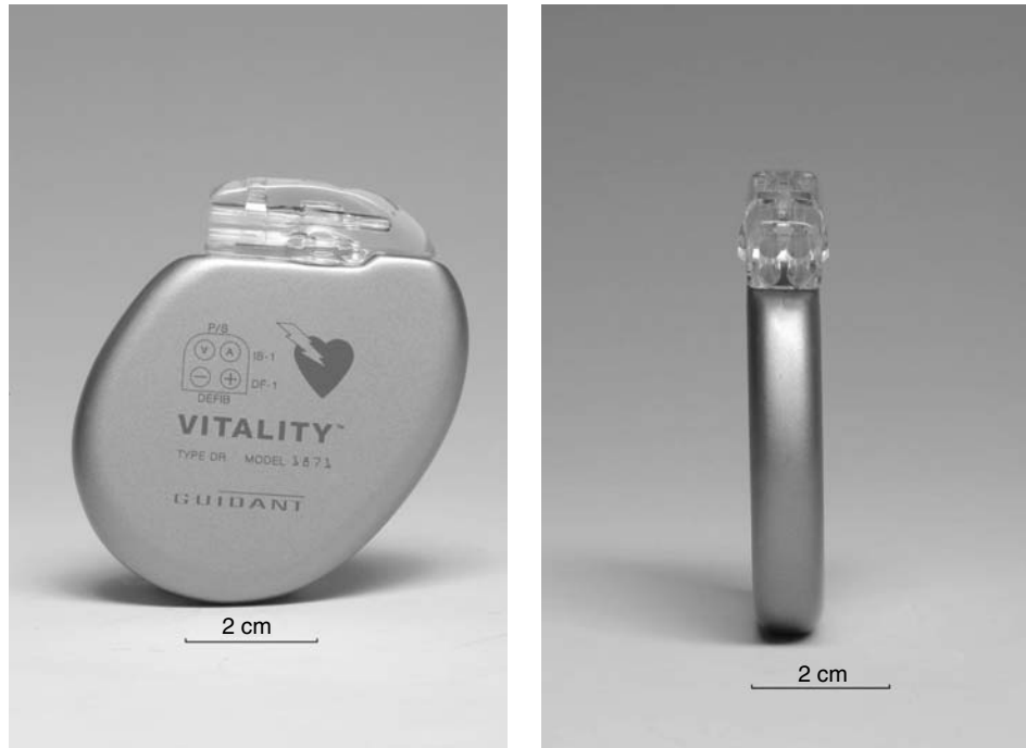
Figure 7 Implantable cardioverter defibrillator
