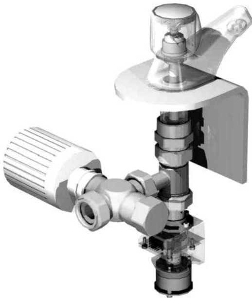
Figure 6 Diagram of the tap developed to enable the water supply to be turned off without taking control away from the user
