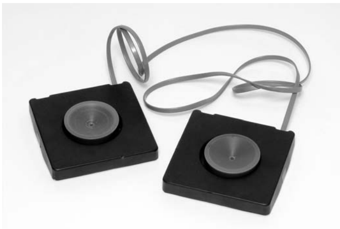
Figure 3 A bed-occupancy sensor that fits under a bed leg
