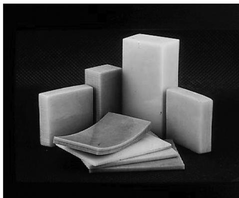
Figure 2. Samples of various CIPP sleeves after curing.
