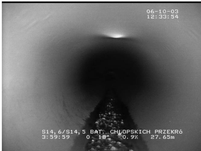
Figure 3. Single point dent in the PVC-U pipe (photograph by the author).
