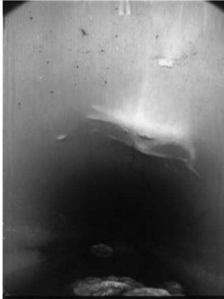
Figure 6. Surface dent in the PVC-U pipe (photograph by the author).
