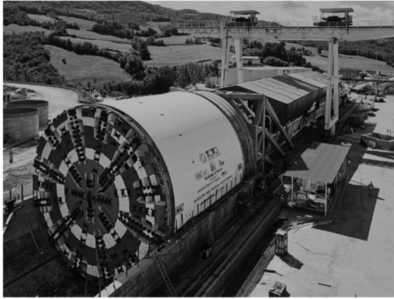
Figure 3. Galleria Sparvo road tunnel – 15.62 m diameter EBP Shield.
