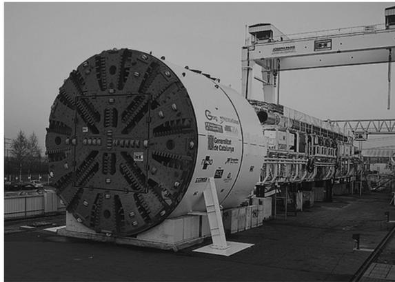
Figure 2. Metro Line 9 Barcelona: 12.06 meter diameter EPB Shield for variable geological conditions.
