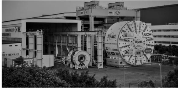
Figure 5. Supersize TBM for TM-CLKL, Mixshield  $\varnothing$ 17.6 m diameter.
