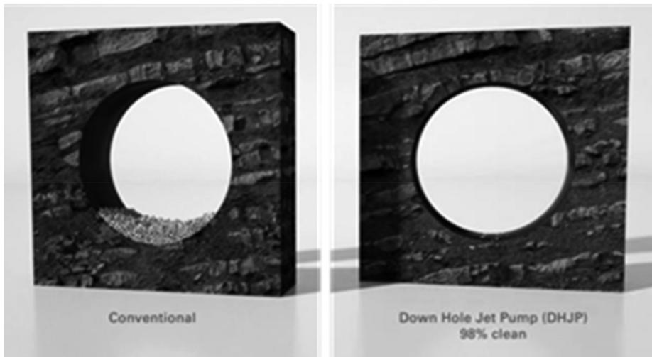
Figure 4. Settlement of cuttings in the borehole with/without the use of the Down Hole Jet Pump.
