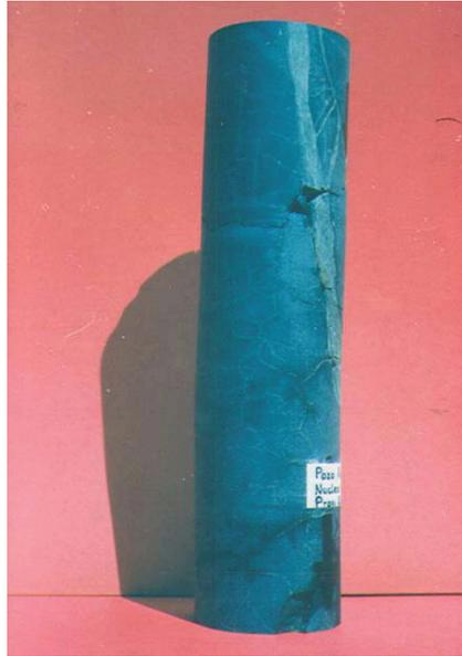
Figure 9.20. Rock core (diameter 10 cm) from Los Azufres geothermal field (Mexico) which is crossed by a 1.5 cm wide sealed fault and a network of fractures with openings of about 0.1 cm.
