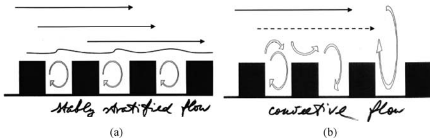
Fig. 7.1 Schematic demonstration of the stability dependence of the roughness length: (a) for stably stratified flows (b) for convective flows
