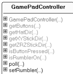
Figure 11-10. Class diagram for GamePadController
