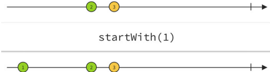
Figure 2-11. A marble diagram of the startWith operator
