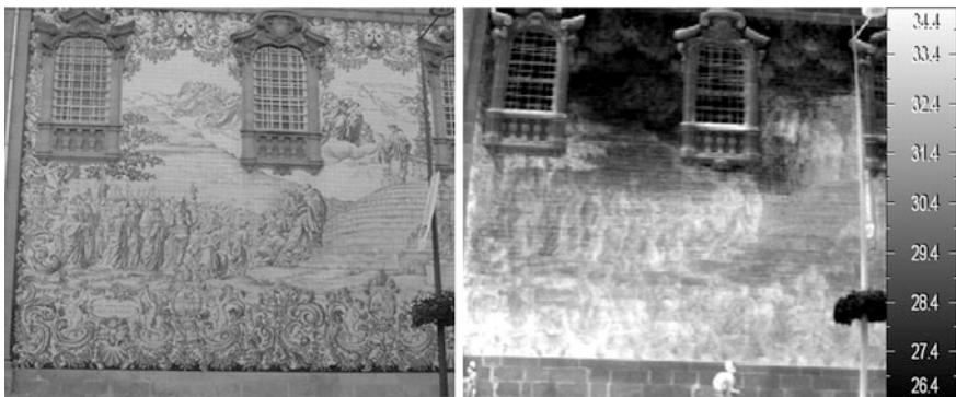
Fig. 1 Visible image and thermogram of the Carmo Church's façade covered with "azulejos" (ceramic tile) in Porto, Portugal
