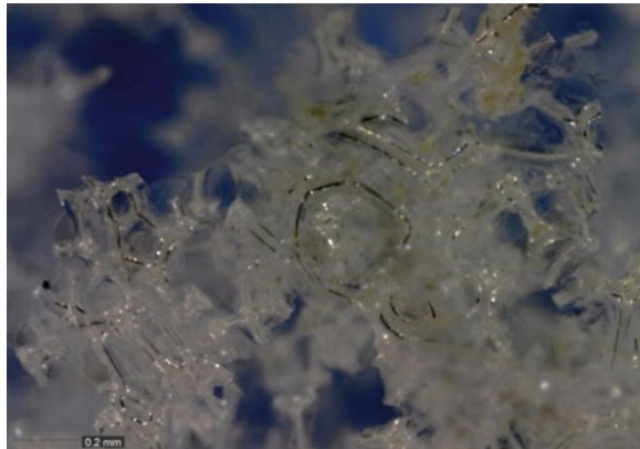
Fig. 6 Detail view of PUR grain fr. 0/4 mm, scaled up 206 time
