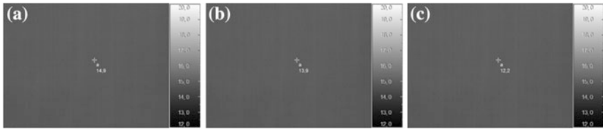
Fig. 4 Thermograms of lime stone specimen obtained with different emissivities: a \epsilon = 1.00 , T_{\text{measured}} = 14.9 \text{ }^\circ\text{C} . b \epsilon = 0.80 , T_{\text{measured}} = 13.9 \text{ }^\circ\text{C} . c \epsilon = 0.60 , T_{\text{measured}} = 12.2 \text{ }^\circ\text{C}
