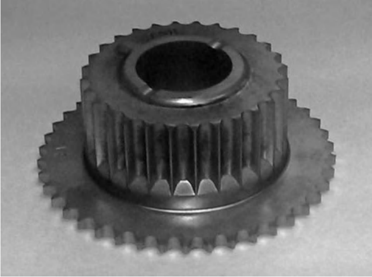
Figure 4.2. A green part as it comes from the press.
