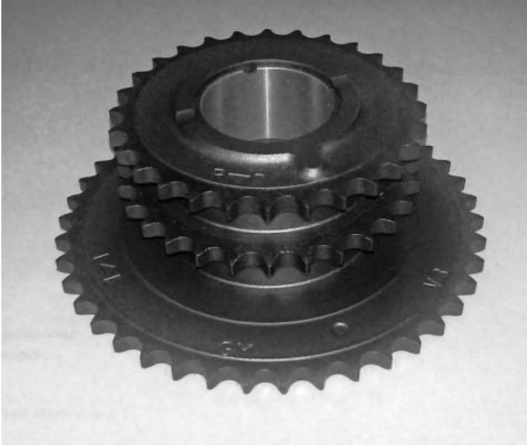
Figure 4.3. A completed part before a rust-preventative treatment is applied.
