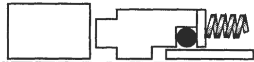
Figure 13-45. A flexible stator with the wear face on the stator.
