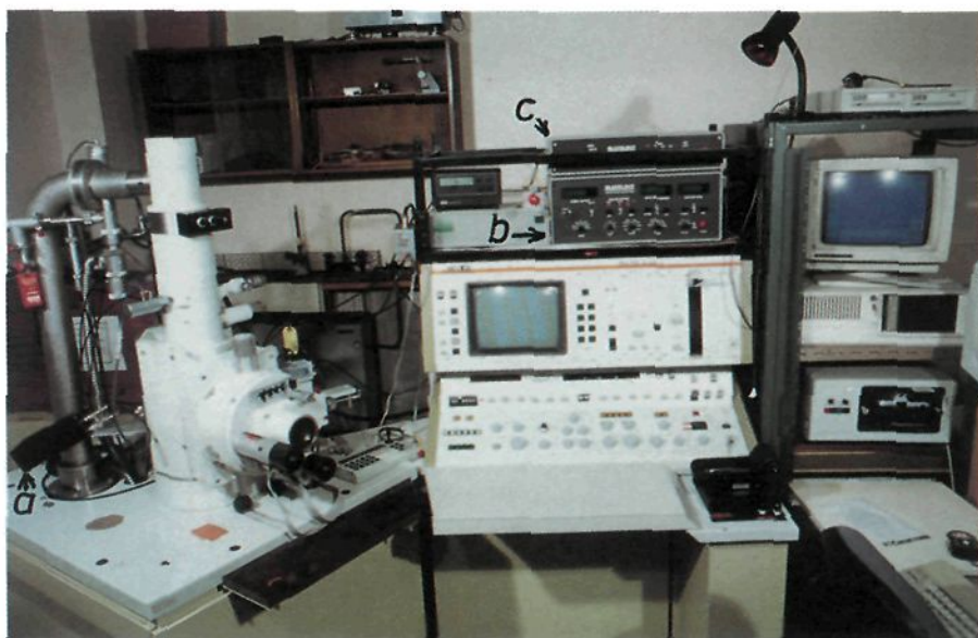
Fig. 18. The SEM and EBIC system. (a) is the head amplifier, (b) the main control unit and (c) is the computer interface module of the EBIC system.
