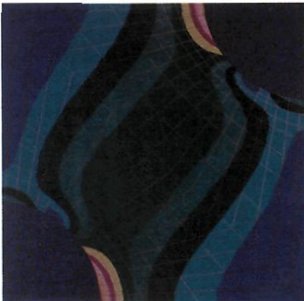
Fig. 10. A computer-generated model of the deformation behaviour of a rubber-toughened epoxy adhesive. The finite-element analysis shows two (one-quarter) spherical rubber particles. The material between the rubber particles is the epoxy adhesive. The green-coloured band represents the development of a plastic shear band in the epoxy polymer — initiated by, and running between, the rubber particles. (The adhesive is being loaded vertically.)
