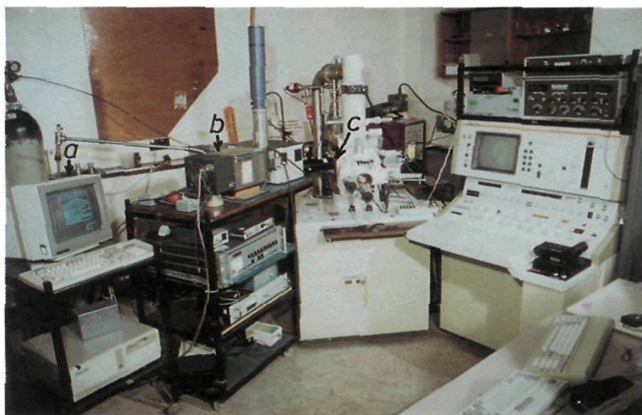
Fig. 20. The CL system. The trolleys at the left hold (a) the control and data logging computer, (b) the CL monochromator system that we developed and, mounted on the side port of the scanning electron microscope, (c) is the Oxford Instruments liquid helium cryostat and CL collection stage unit.
