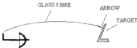
Fig. 19. Production of glass fibres by the method developed by Boys. 17
