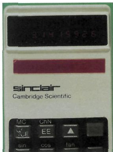
Fig. 26. A Sinclair Cambridge hand calculator showing the red GaP LED \alpha -numeric display.
