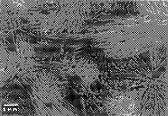
Fig. 32. Microstructure of Apoceram bioactive glass-ceramic (the crystalline phase is light coloured and the residual glass is dark).
