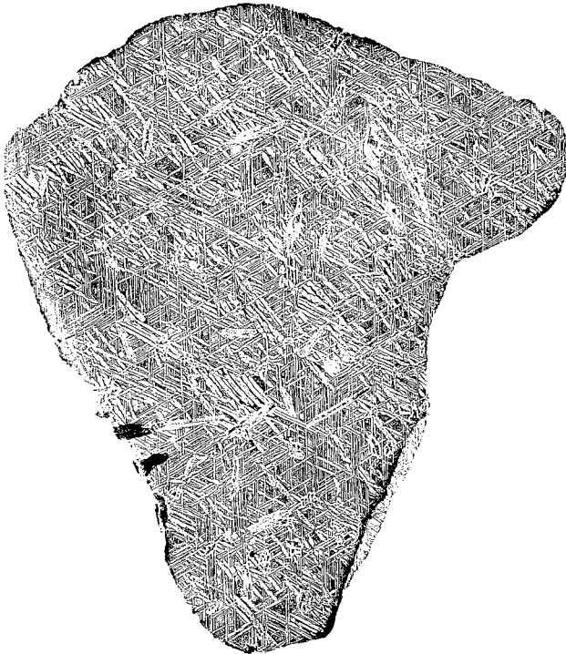
Fig. 2. An imprint from the polished and etched cross section through a meteorite produced in 1813. (Ref. 24, reproduced with permission).
