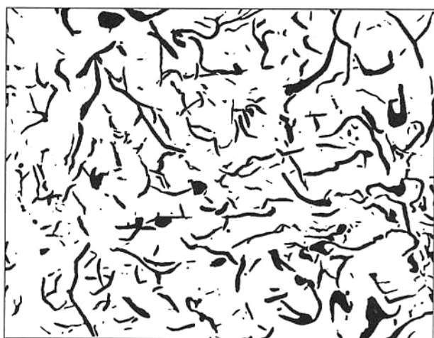
Fig. 4.26. Graphite in gray cast iron (top) is an ideal example of particles which are easy to detect by binarization (bottom).
