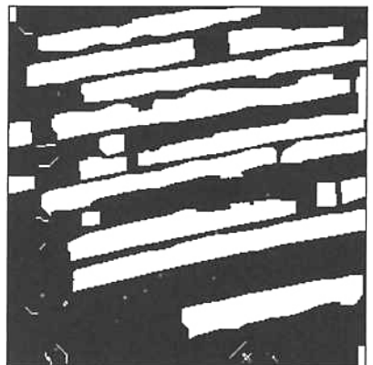
Fig. 4.43. Analysis of the fracture surface of a carbon-epoxy composite: initial image (a), its initial (b) and filtered (c) Fourier spectrum, inverse Fourier transformation (d), Fourier filtered fibers (e) and detected fibers (f).
