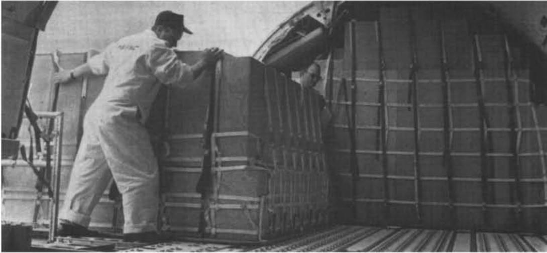
Masses of ball transfer units in airplane floor make it easy to shove cargo loads in any direction.
