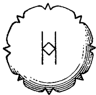
Fig. 15—Arched-nut attachment requires no machining. Nut is first rammed into tube; tightening of screw forces barbs into metal for positive anchorage.
