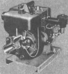
DIFFUSER priming method here does not return liquid to suction side of the pump
