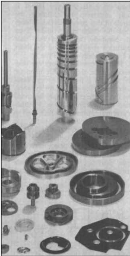
New technique produces wide variety of shapes, including barrel and cup cams.
