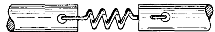
Fig. 13—Spring joins two rods or tubes. Members are not limited in axial motion or rotation except by spring strength.
