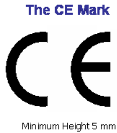
Figure 7.13 The standard CE mark signifying a claim to conform to relevant directives
