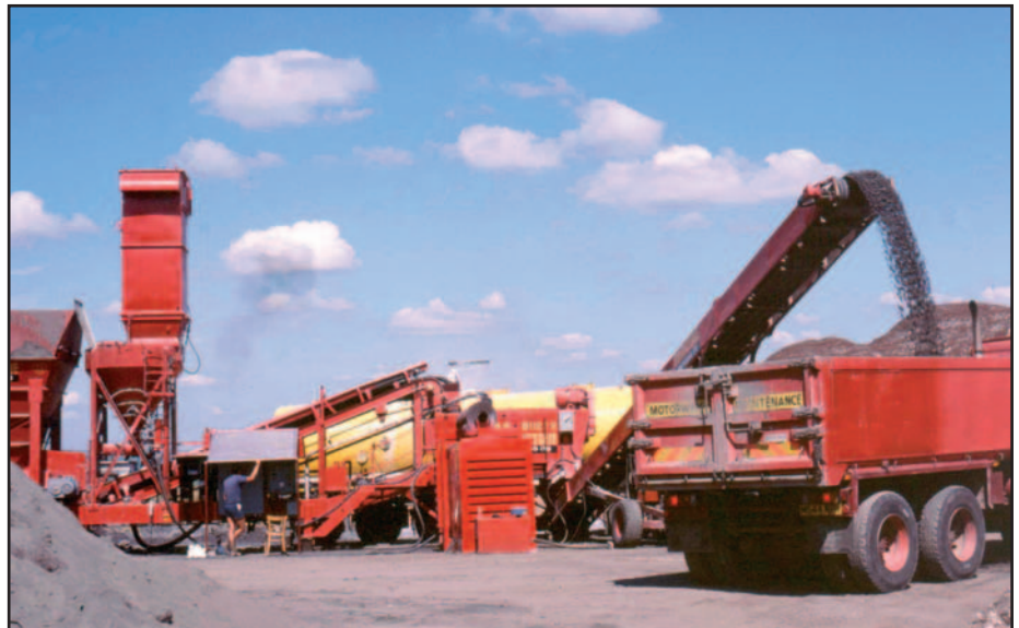
Figure 2 Stationary-mixing plant for the mix-in-place method of construction.
