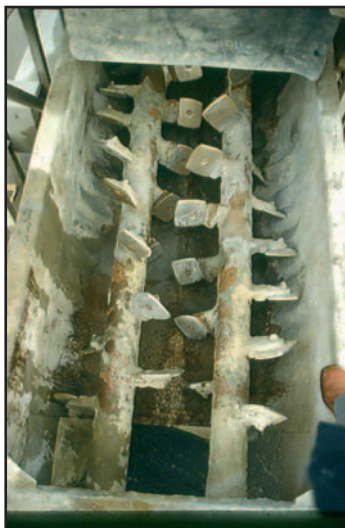
Below: Figure 18 A close-up of a continuous pug-mill mixer showing the mixing trough, shafts and blades.
