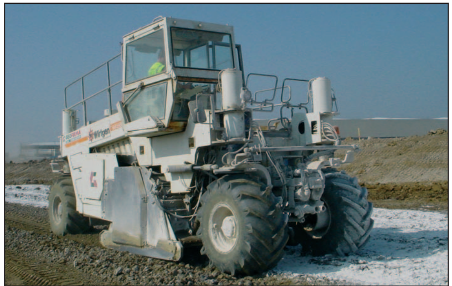
Right: Figure 16 Rotovator with rotor mounted between axles. These types of rotovators can be 'fitted' with an internal powder-storage hopper, which dispenses the blanket of powder on the ground about 300mm in front of the rotor hood.
