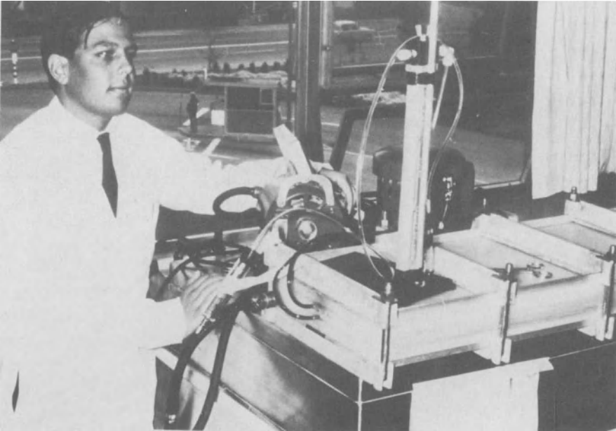
Figure 10. Robin Eady learning his trade as a hemodialysis technician in the spring of 1963. An early Western Gear Kiil dialyzer is in the foreground.
