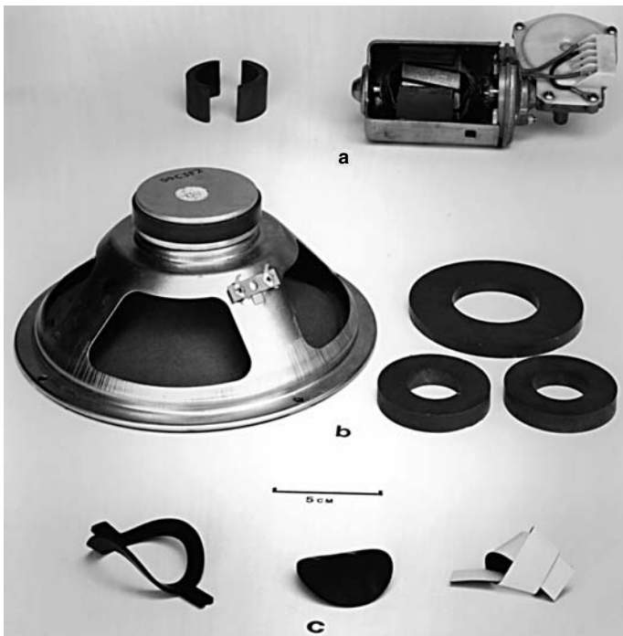
Fig. 9.59 Hard ferrite components: (a) windscreen wiper motor and ferrite segments; (b) loudspeaker and field magnets; (c) hard ferrite-polymer composites. (Perspective size distortion; identification letters are the same actual size.)
