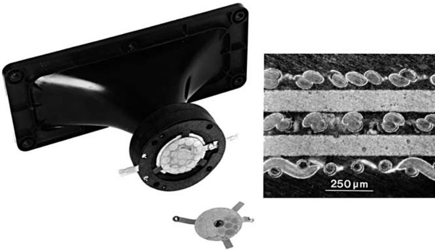
Fig. 6.33 Hi-fi ‘tweeter’ showing ceramic bimorph plate element. Inset, cross-section of element showing piezoceramic plates sandwiched between metallized glass fibre mesh.
