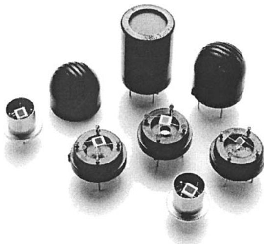
Fig. 4.50 A selection of commercial gas sensors. The alumina tile carrying the sensor is approximately 3 \times 3 \text{ mm}^2 . An activated charcoal filter may be mounted inside the top of the housing. (Courtesy of City Technology Ltd.)
