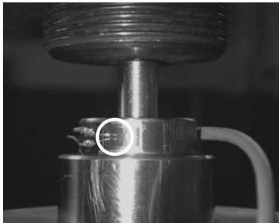
Fig. 14 Close-up of a tapered specimen during assembly showing the collar instrumented with an electrical-resistance strain gauge (circled)
