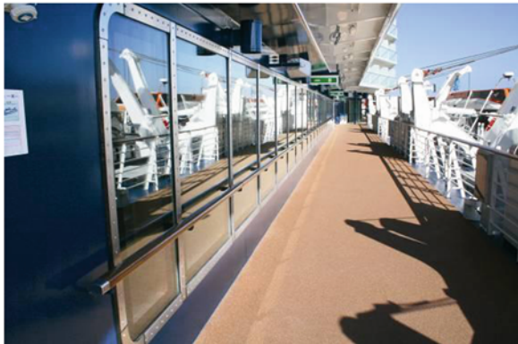
Fig. 3 Bonded windows for cruise ships: a glass façade showing (small) retaining frames, b fire protective glazing with substantial retaining frames (with permission from Brombach + Gess)
