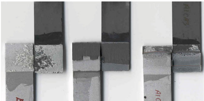
Fig. 9 Failure surfaces of CFRP–aluminium lap joints ( left : LM adhesive only; middle : HM adhesive only; right : mixed-adhesive)
