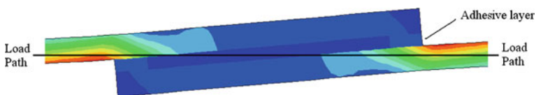
Fig. 1 Principal stress distribution in the adherends of a lap joint loaded in tension
