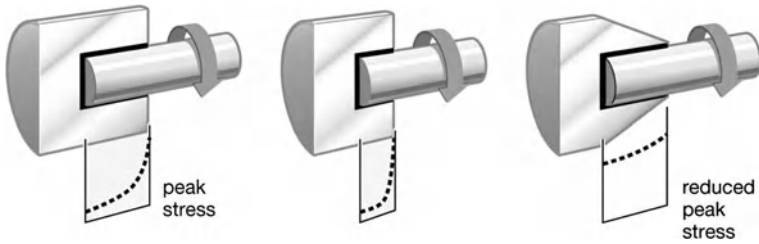
Fig. 8 Stress distribution across bond
