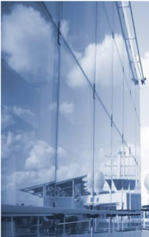
Fig. 3 Bonded windows for cruise ships: a glass façade showing (small) retaining frames, b fire protective glazing with substantial retaining frames (with permission from Brombach + Gess)
