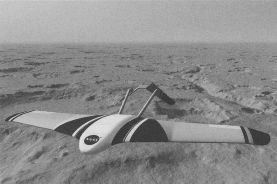
FIGURE 9.4 ARES, a NASA concept for a small plane that is to explore Mars from the air. [NASA]
