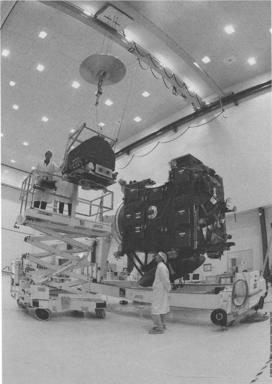
FIGURE 4.3 Cleanrooms can be very large. Here the Rosetta comet lander is hoisted on top of its mother spacecraft in ESA's test area. [ESA]
