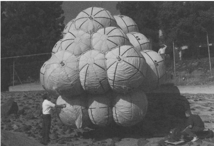
FIGURE 2.8 Airbags are used to protect a lander when it hits the surface of a planet. The landing is however much rougher than with a rocket brake system [NASA]
