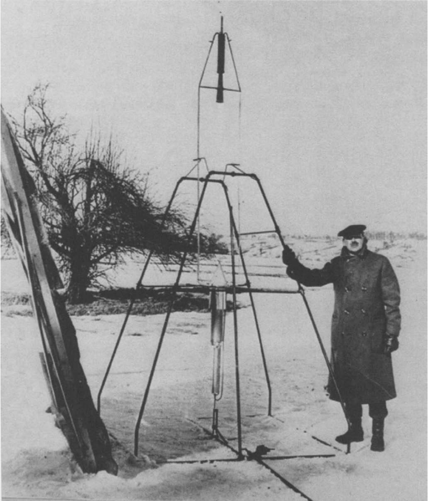
FIGURE 1.2 Dr Robert H. Goddard with the world's first liquid propellant rocket, which he launched in 1926. Unlike in modern rockets, the nozzle is on top. [NASA]
