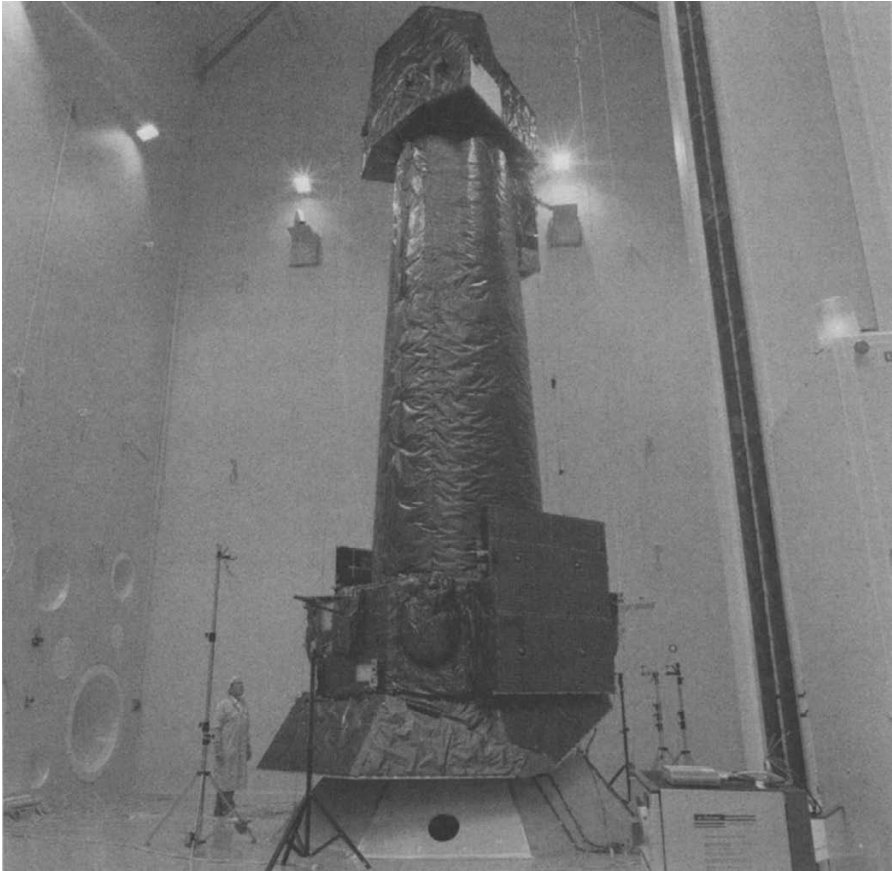
FIGURE 4.8 ESA's XMM space telescope inside the giant Large European Acoustic Facility, where the acoustic violence of a rocket launch can be simulated. [ESA]
