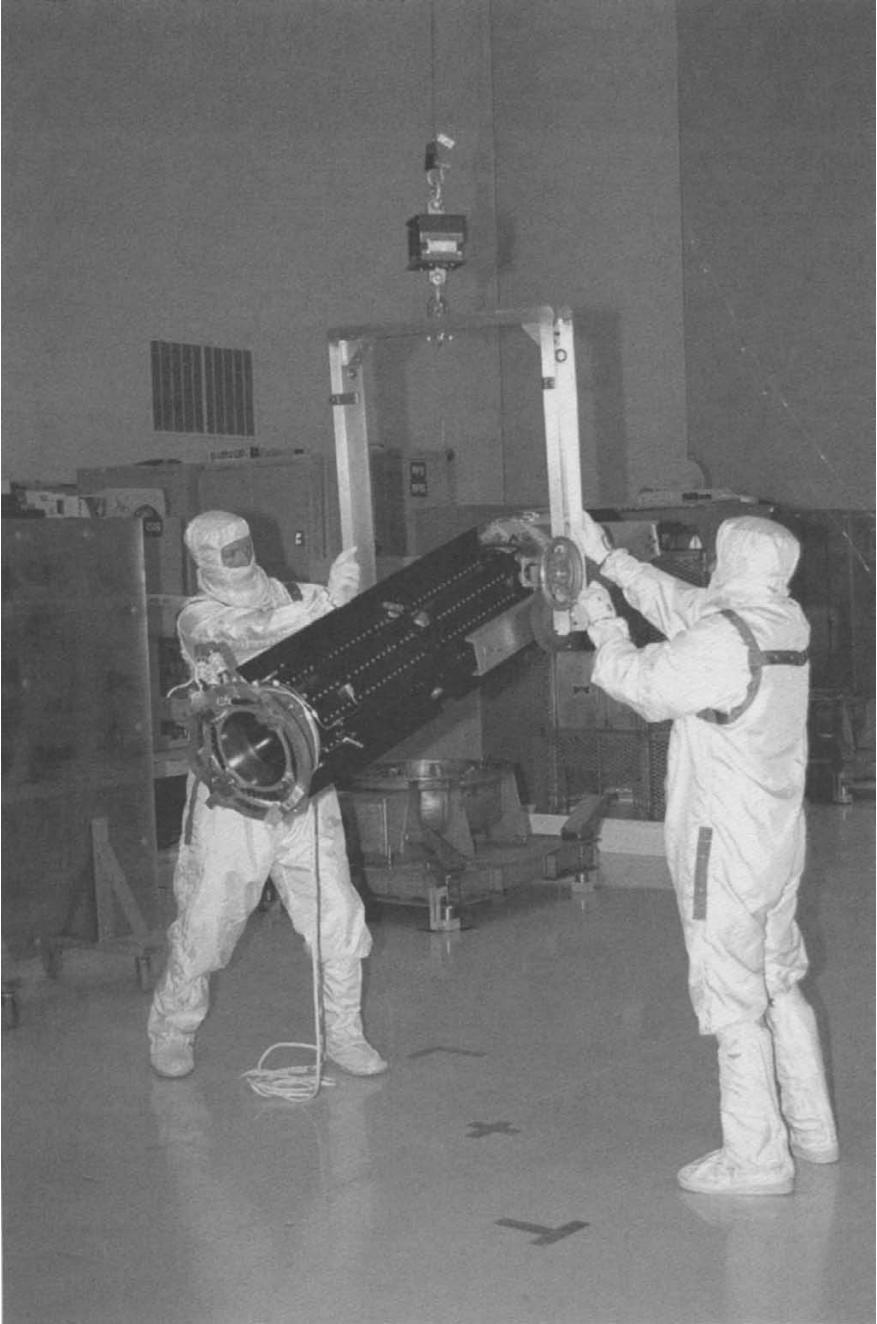
FIGURE 3.4 One of the RTGs used on Cassini just before integration with the spacecraft. [NASA]
