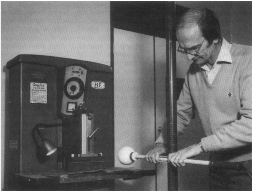
Figure 4.4 Characterisation of electric fields from a radio frequency PVC welding machine
