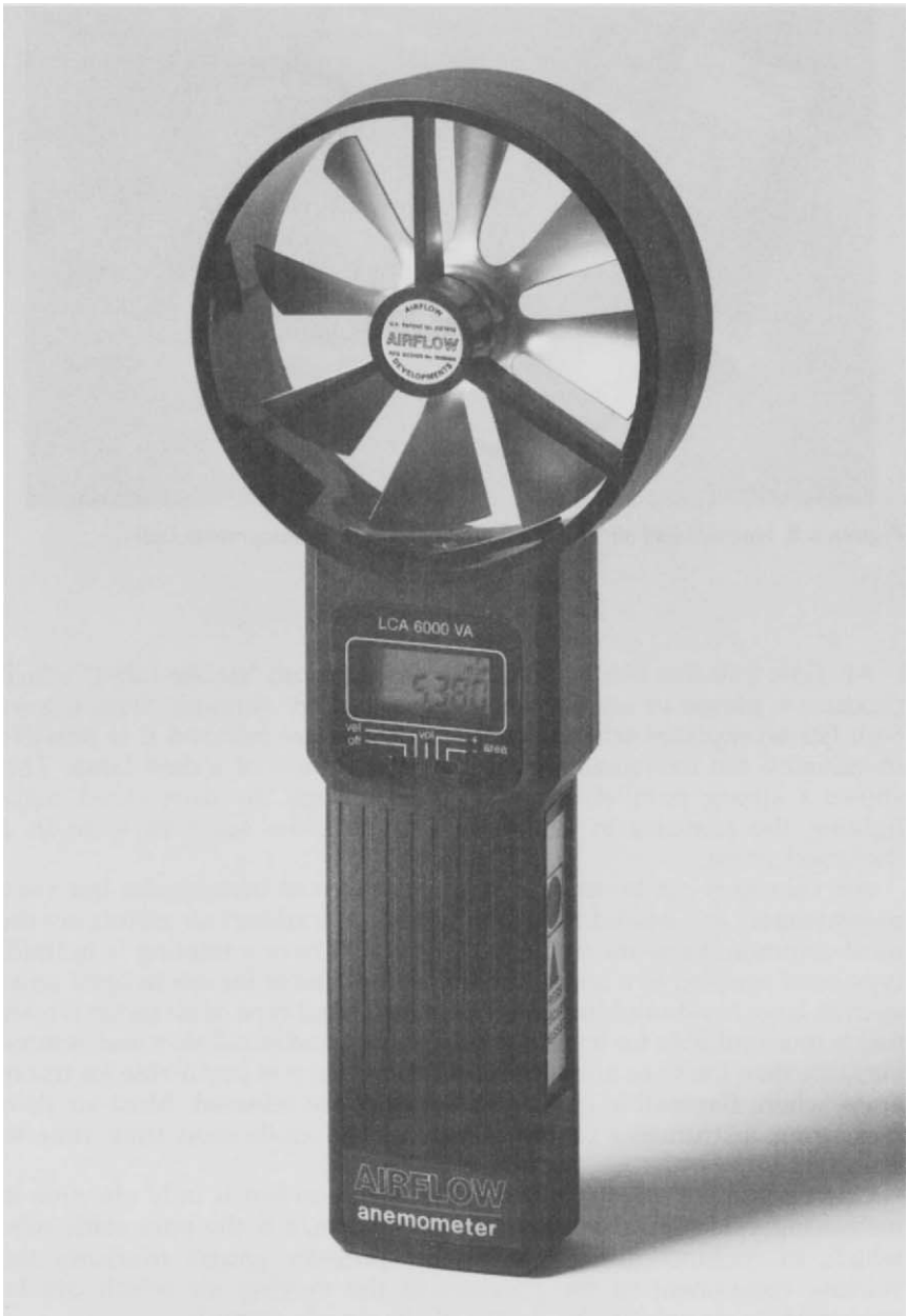
Figure 6.7 Vane anemometer. (Courtesy Air Flow Developments Ltd)
