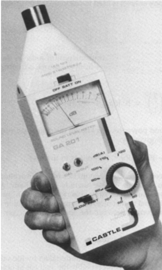
Figure 5.6 Industrial hand-held sound level meter. (Courtesy General Acoustics Ltd)
