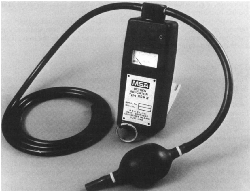
Figure 3.11 Portable oxygen analyser. (Courtesy M.S.A. Ltd)
