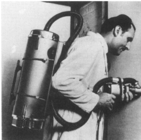
Figure 6.4 High velocity low volume extractor. (Courtesy BVC Ltd)
