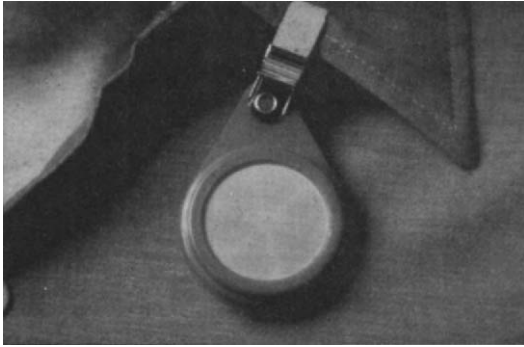
Figure 3.6 Passive monitoring badge. (Courtesy of 3M United Kingdom plc)
