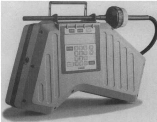
Figure 3.8 Portable infrared gas analyser. (Courtesy Foxboro Analytical Ltd)
