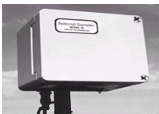
FIG. 6.1. Rotating impaction sampler: Rotorod sampler model 40 (Sampling Technologies, Minnetonka, MN). (Courtesy of Medical Media Service, Wm. Middleton Memorial Veteran's Hospital, Madison, WI.)
