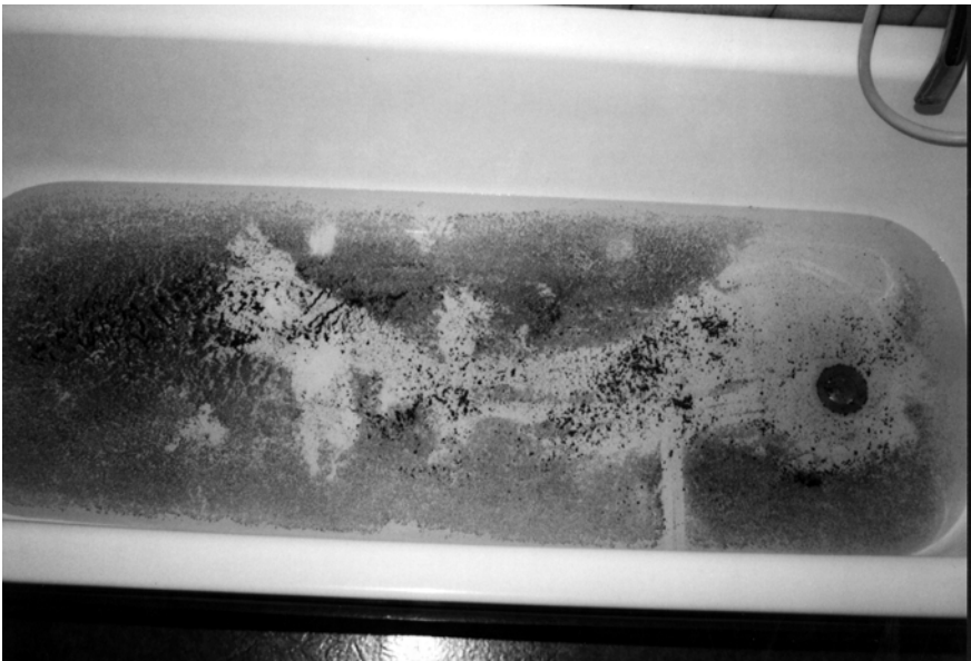
Figure 7.10 Tap water contaminated with iron and manganese
