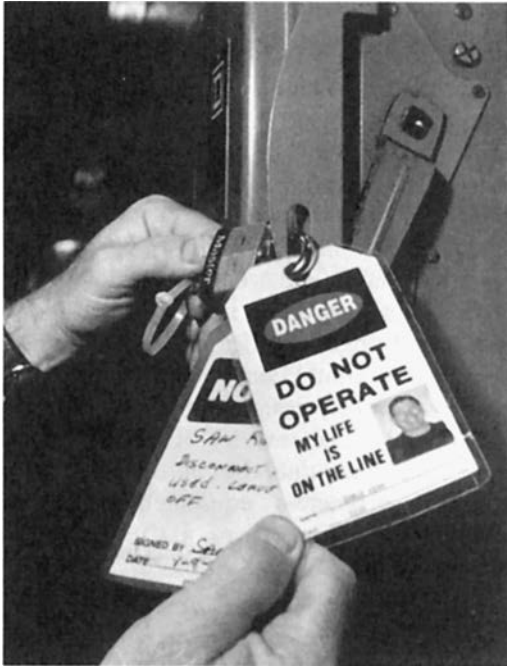
FIGURE 10-4 • Three workers' locks are in place on this machine power switch. All must remove their locks before the machine can be started. (From Occupational Safety and Health Administration. Concepts and techniques of machine guarding. Publication No. OSHA 3067. Washington, DC: Occupational Safety and Health Administration, 1980:60.)
