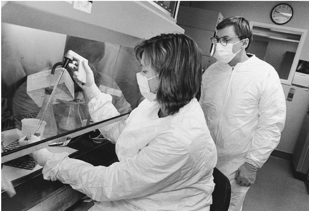
FIGURE 15-2 ● Workers in an HIV/AIDS laboratory are at risk of acquiring HIV infection. This photograph shows HIV/AIDS laboratory workers using personnel protective equipment and exhaust ventilation under a hood. (Photograph by Earl Dotter.)
