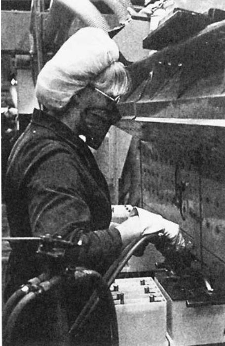
FIGURE 29-2 • Adequate control of lead exposure for all workers requires a high level of engineering control and may also include the need for personal protective equipment. Because U.S. law prohibits exclusion of pregnant women from lead work, controls must be sufficient to protect the fetus as well. (From Zenz C. Occupational medicine: Principles and practical applications. Chicago: Year Book, 1975. Reproduced with permission.)
