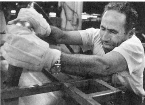
FIGURE 11-7 ● This job requires exerting high hand force with elevated shoulders, increasing the risk of shoulder and upper extremity injuries. (Photograph by Earl Dotter.)
