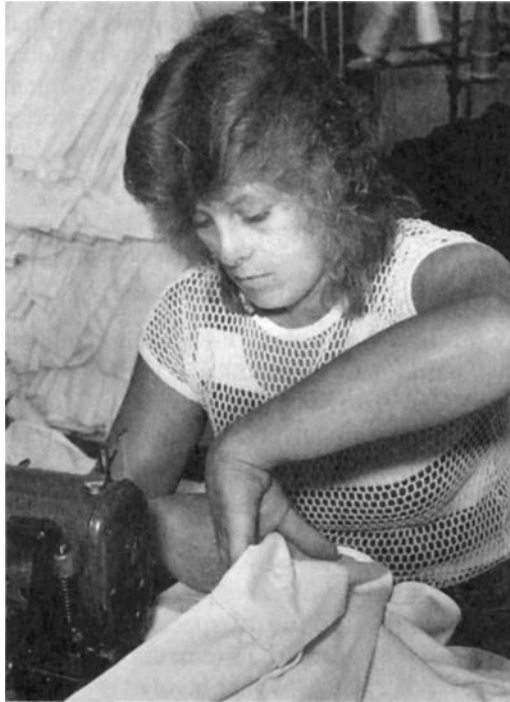
FIGURE 11-8 • Garment workers must repetitively use awkward wrist and shoulder postures when operating sewing machines. (Photograph by Earl Dotter.)
