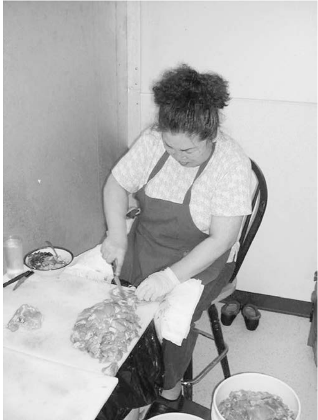
FIGURE 23-2 ● Woman in Nicaragua cutting meat. A high degree of hand force and frequent repetition combine to make this a high-risk job for development of carpal tunnel syndrome and tendonitis. In addition, this woman faces the potential hazards of cuts and neck strain. (Photograph by Barbara Silverstein.)
