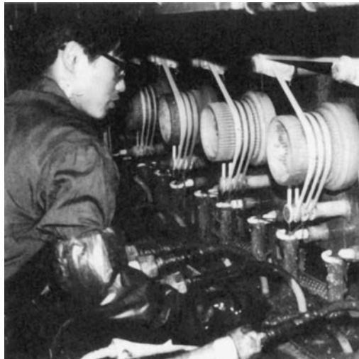
FIGURE 30-1 ● A worker tends machines that spool rayon thread from carbon disulfide. Worker exposure to carbon disulfide was high until this process was enclosed, which reduced worker exposure and, by recycling of the carbon disulfide, saved the company a substantial amount of money (Liang YX, Qu DZ. Cost benefit analysis of the recovery of carbon disulfide in the manufacturing of viscose rayon. Scand J Work Environ Health 1985;11(Suppl. 4):60–3. Photograph by Barry S. Levy.)
