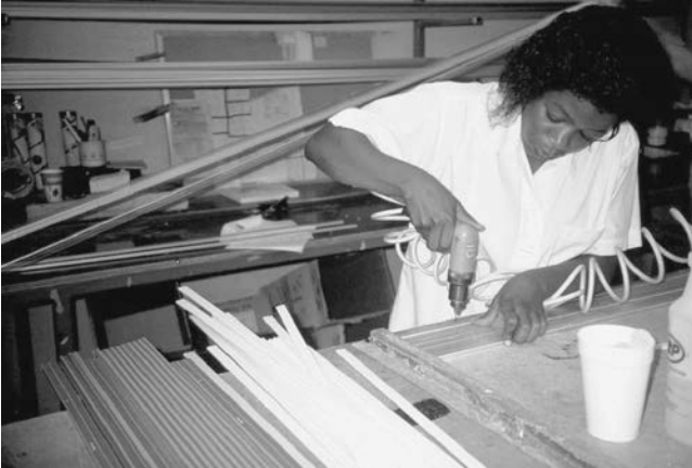
FIGURE 23-3 • In jobs like this, reducing the load on the wrist, elbow, and shoulder can be accomplished by one or more of the following three methods: changing the tool, reorienting it (from vertical to horizontal, or vice versa), and changing the height of the work station—either elevating the worker or lowering the piece being worked on. (Courtesy of WISHA [Washington Industrial Safety and Health Act] Services Demonstration Project.)
