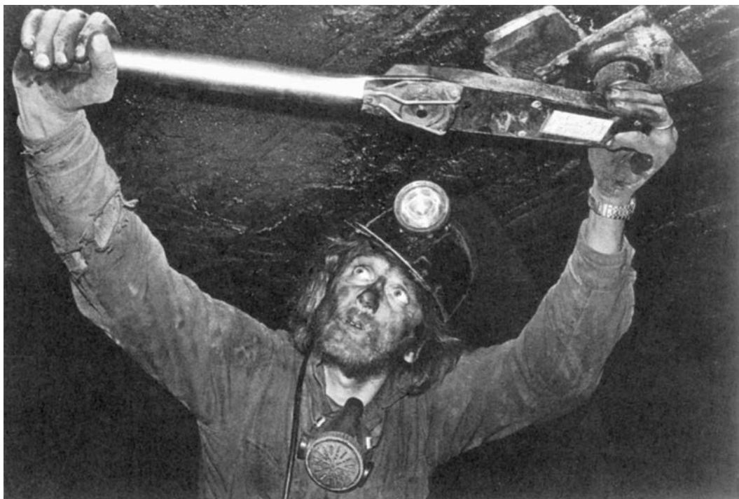
FIGURE 1-2 • Roof bolting in coal mines is essential to prevent roofs from collapsing. Miners, like this man testing the mine roof support bolts in a Pennsylvania coal mine, face many other injury risks as well as exposure to hazardous dusts, gases, and other substances. (Photograph by Earl Dotter.)
