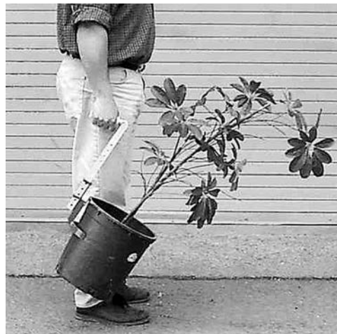
FIGURE 32-2 • (A) Picking up and carrying large potted plants in this manner increases the risk of low back and upper extremity injuries. (B) This device, used as an ergonomic intervention for nursery workers, reduces the need to bend in order to pick up potted plants; it also has a handle designed to decrease stress on the upper extremities. (Courtesy of University of California Davis.)
