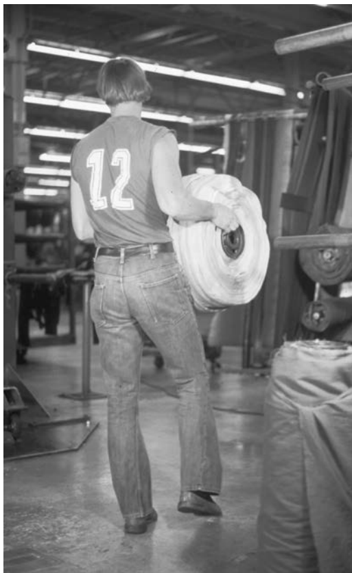
FIGURE 11-2 • The load carried by this worker exceeds 50 kg (110 lb). A mechanical-assist device such as an overhead hoist would reduce the risk of back injuries on this job.
