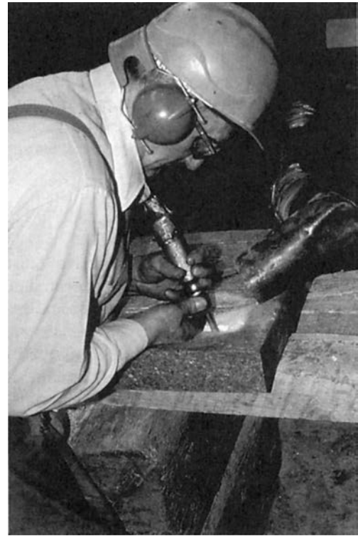
FIGURE 9-4 • Local exhaust ventilation successfully captures dust produced by stone cutting. (From W. A. Burgess, Harvard School of Public Health, Boston, Massachusetts.)
