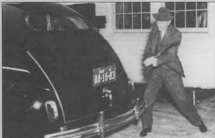
Henry Ford demonstrates the durability of automobile components made from soybeans by striking the trunk of a car with an axe. (From the collections of Henry Ford Museum & Greenfield Village.)
