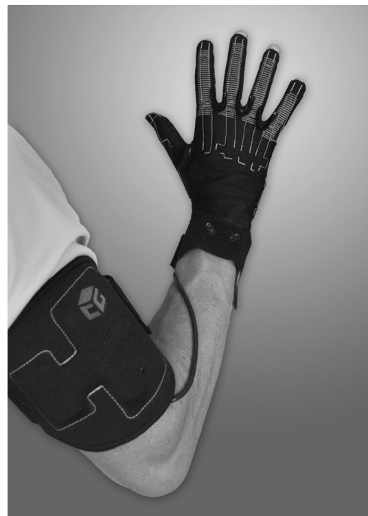
Fig. 34.3 CyberGlove III, including 18 to 20 sensors. With kind permission of CyberGlove Systems LLC.
