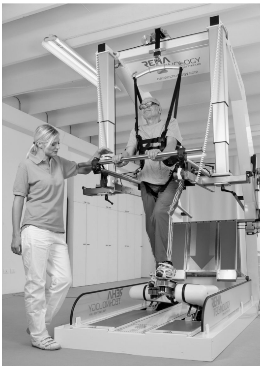
Fig. 32.3 The end-effector based G-EO training robot supporting users in practising walking and stair climbing.
