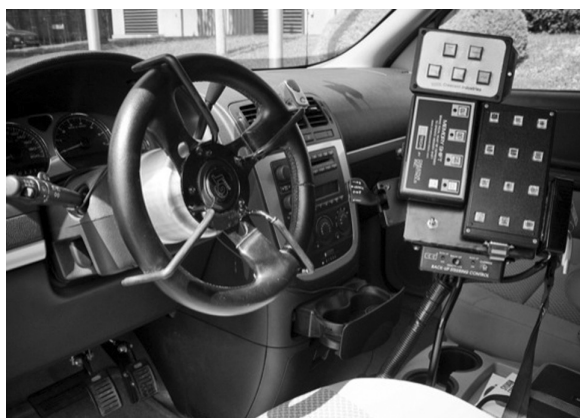
Fig. 33.5 Adaptation of the primary controls of a vehicle. Constance-Lethbridge Rehabilitation Centre ( http://www.constance-lethbridge.qc.ca/ )
