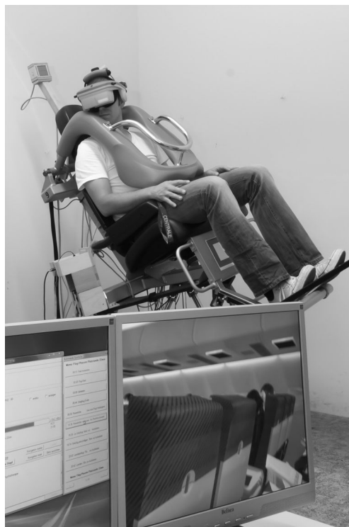
Fig. 34.11 Simulator for the treatment of aviophobia (fear of flying). Courtesy of Prof. A. Mühlberger, University of Würzburg, Germany.
