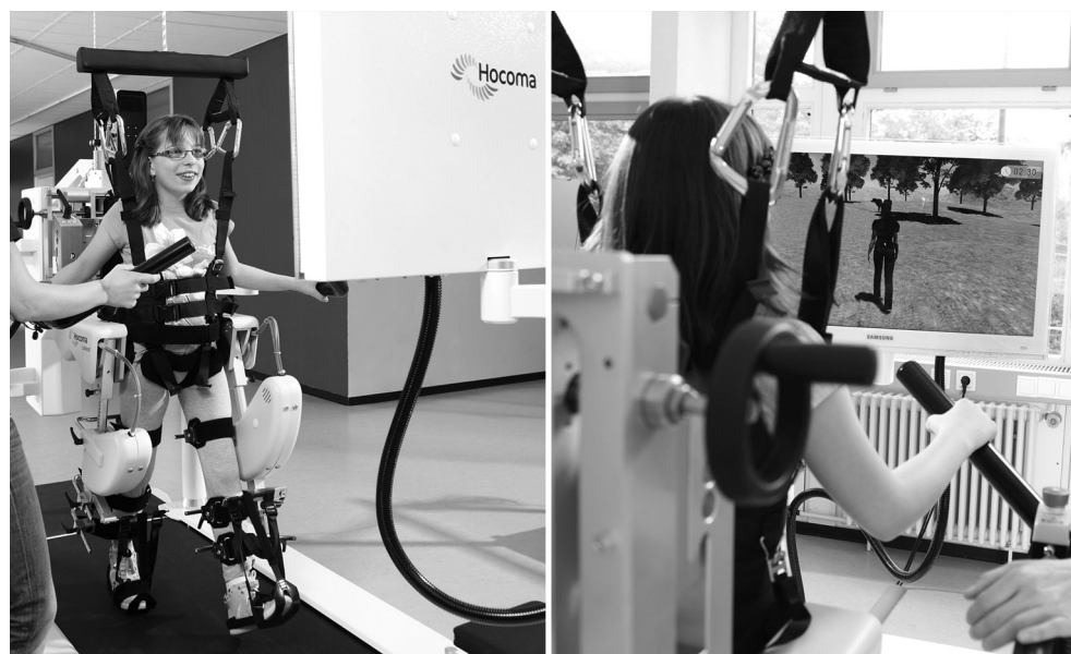
Fig. 32.6 Driven gait orthosis ‘LokomatPro’ with pediatric module and virtual reality. With kind permission of Hocoma AG, Volketswil, Switzerland and SRH Hospital Neckargemünd, Germany.
