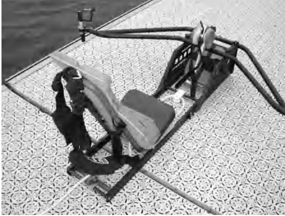
Figure 20.3. The Alden (16 & 18), ( www.rowalden.com ), detachable state room with modified seat, padded shoulder straps and bungee cord, pulley and cam cleat to allow adjustment of bungee cord tension. The telescopic leg stabiliser is similar to that used on the indoor rower.
