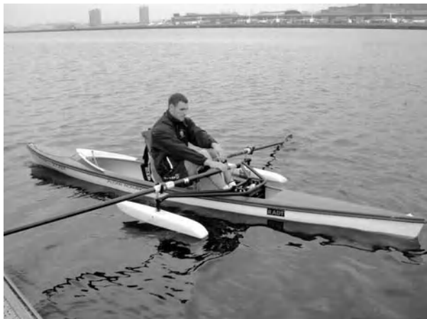
Figure 20.6. Subject 6 in the adapted Alden 16 shell. The floats mounted below the oarlocks prevent capsizing.
