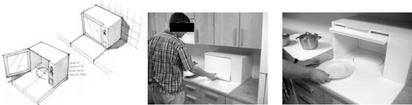
Figure 12.6. Microwave: a slide-in unit into the notched counter surface places the turntable at the counter line. This configuration enables older people with arthritic hands to slide hot dishes and liquids safely from within the microwave to the counter surface unlike contemporary microwaves where the lip of the turntable and transitioning to the counter top often causes spills.
