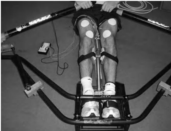
Figure 20.4. The FES rowing simulator, comprising an Alden boat stateroom fitted with hydraulic cylinders for laboratory training and development
