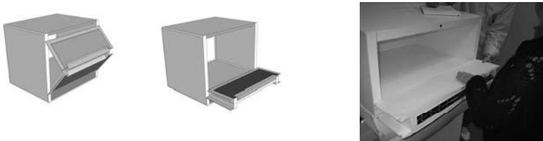
Figure 12.5. Wall oven: a split folding door allows hot interior surfaces to mate, thereby minimising reach-over distance and accidental burns. The door opens at the counter line to provide a transition surface.
