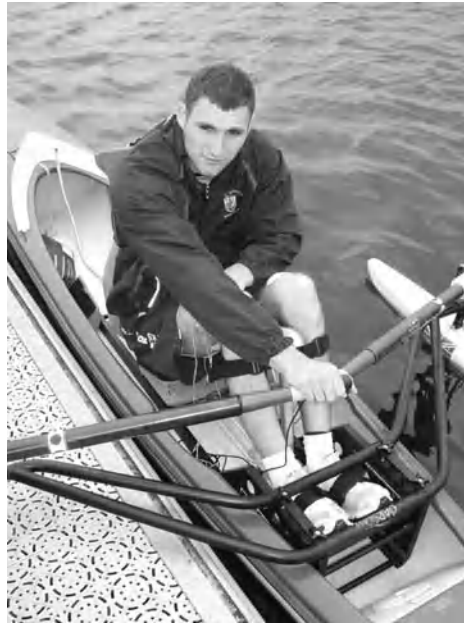
Figure 20.5. The adapted stateroom module shown in Figure 20.3 is shown installed into the Alden 16 shell. Subject (6) is shown dockside with the leg stabiliser in place, testing the control switch fixed to the oar handle.
