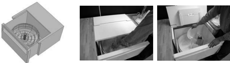
Figure 12.7. Dishwasher: a 19” tall and 30” wide under-counter pullout drawer, with turntable dish rack and counter level hide-away lid. All dishes are accessible through the top lid of the drawer can be pulled out a few inches to gain further access but not encroach completely into the walk area.
