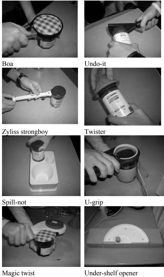
Figure 7.1. Various opening tools used in the testing
