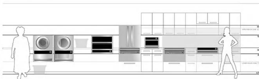
Figure 12.3. The “strike zone” concept illustrated in elevation with appliance suite organised linearly
