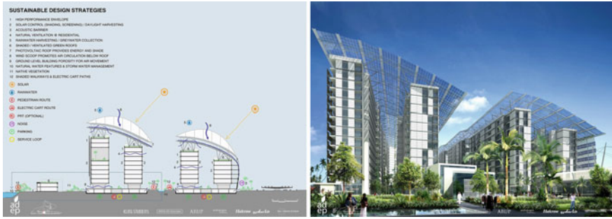
Fig. 4.11 Abu Dhabi Ecological Residential Park—perspective and concept section showing solar canopies (Nader Ardalan)
