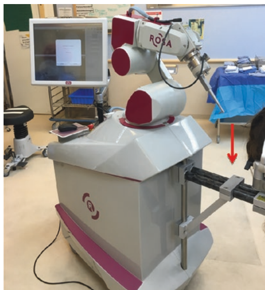
Fig. 13.10 Rosa™ (MedTech Surgical Inc., Newark, NJ). Red arrow showing arm where robot attaches to patient head holder
