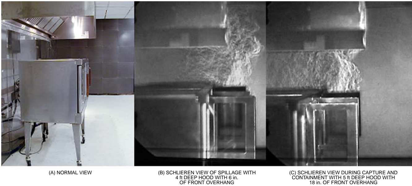
Fig. 10 Three Ovens under Wall-Mounted Canopy Hood at Exhaust Rate of 3400 cfm (Swierczyna et al. 2005)
