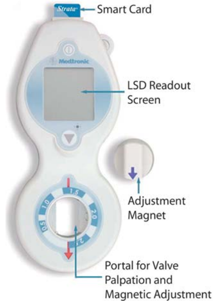
Fig. 2.20. Strata valve programmer (courtesy of Medtronic Neurologic Technologies)
