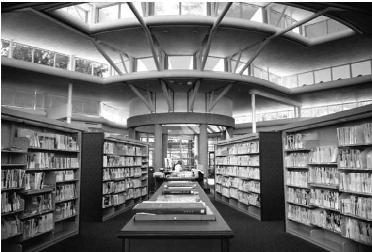
FIGURE 13.3 Boulder, Colorado, Public Library lighted by clerestories and skylights. (Courtesy of Lightforms, Inc.)
