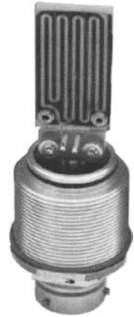
FIGURE 12.12 Photograph of humidity and temperature sensor. (Courtesy of Phys-Chem Scientific Corp., New York. With permission.)
