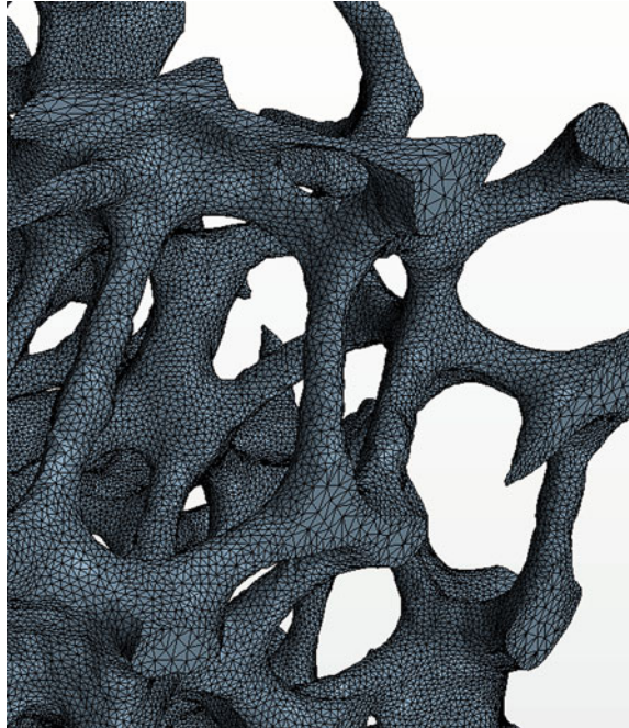
Fig. 1 Foam matrix surface mesh. Sample size: 15 \times 15 \times 15 mm. Volume mesh: about 10 million polyhedral cells
