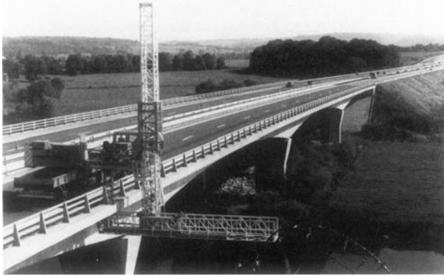
FIGURE 12.9 Scorpion II X-radiography system on prestressed concrete bridge structure. (Photo courtesy of Laboratoire Régional des Ponts-et-Chaussées de BLOIS.)
