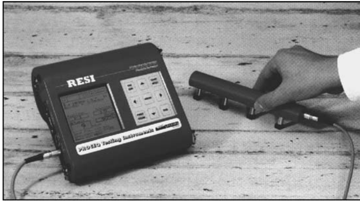
FIGURE 11.13 Example of commercial apparatus to measure concrete resistivity. (Courtesy of Proceq SA.)
