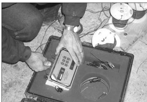
FIGURE 5.15 Example of multichannel maturity meter using thermocouple wires to monitor in-place temperature. (Courtesy of American Engineering Testing, Inc.)
