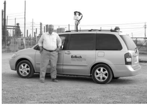
FIGURE 15.3 Infrared thermographic radiometer sensor and optics mounted on a custom-designed mobile van designed to hold the electronic processing and computer enhancement systems.
