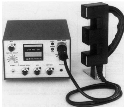
FIGURE 10.3 A meter used to locate reinforcement. Instrument includes a standard probe, a special probe for magnetic concrete, headphones and a spacer block for rebar measurement. (Courtesy of NDT James Instrument Inc.)
