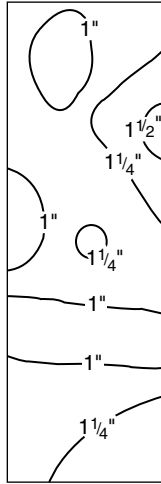
FIGURE 10.4 Depth of concrete cover on a reinforced concrete bridge deck.
