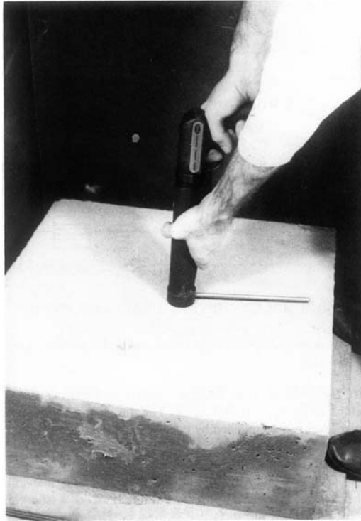
FIGURE 2.3 A view of the Windsor probe in operation: a 600 × 600 × 200-mm slab under test for correlation purposes. (Adapted from Reference 21.)
