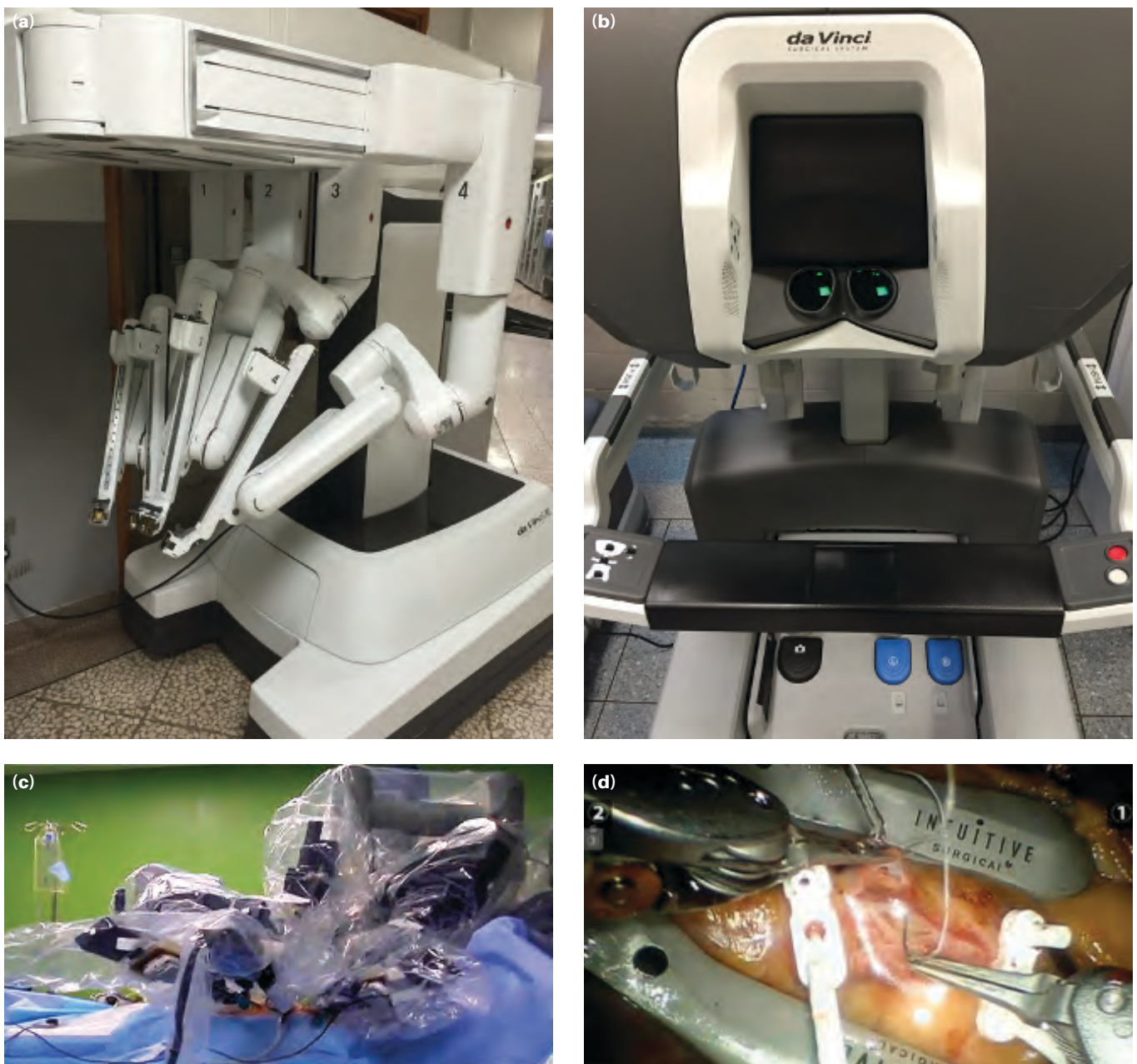
Figure 8.2 (a) The DaVinci Xi system. (b) The surgical console. (c) The robotic arms draped for a robotic coronary artery bypass grafting procedure. (d) Robotic distal coronary anastomosis.
