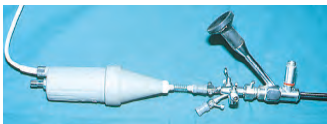
Figure 77.30 An endoscopic ultrasound probe, which is used to fragment bladder or kidney stones.
