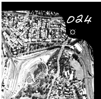
Figure A5.6 Typical fiducial mark on an air survey photograph
