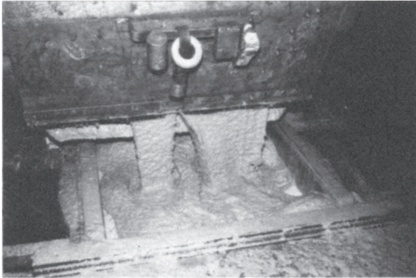
Fig. 6.27. Secondary hopper feed.
