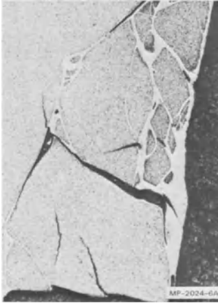
Figure 9. Network of White-Etching Shear Bands and Associated Cracks Near a Ballistic Performance in ESR 4340 Steel
