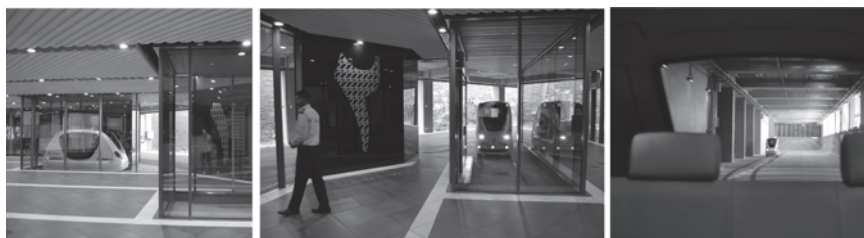
Figure 16.6 Personal rapid transit in Masdar City's undercroft. Instead of 80 docking stations spread underneath the city's surface as originally planned, only one station connects the car park with the Masdar Institute. (Source: authors.)
