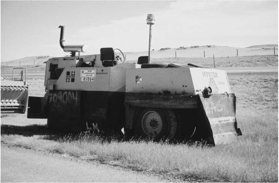
Plate 9.31 Pneumatic roller used for chip seals.
