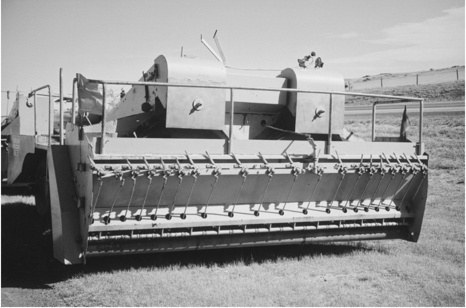
Plate 9.30 Aggregate distribution gates.
