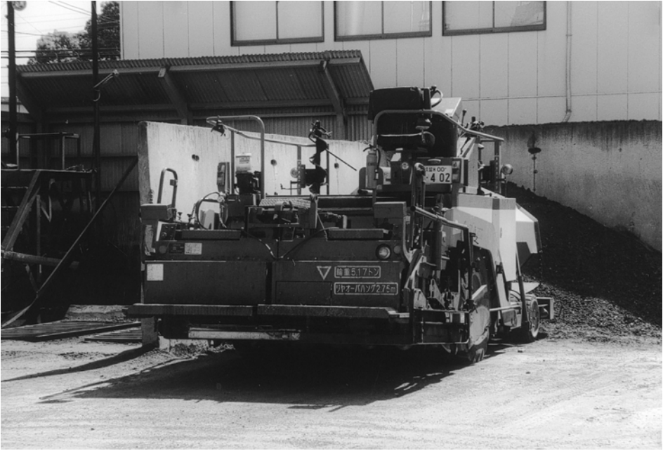
Plate 6.33 Floating screed, capable of variable widths and crowns.
