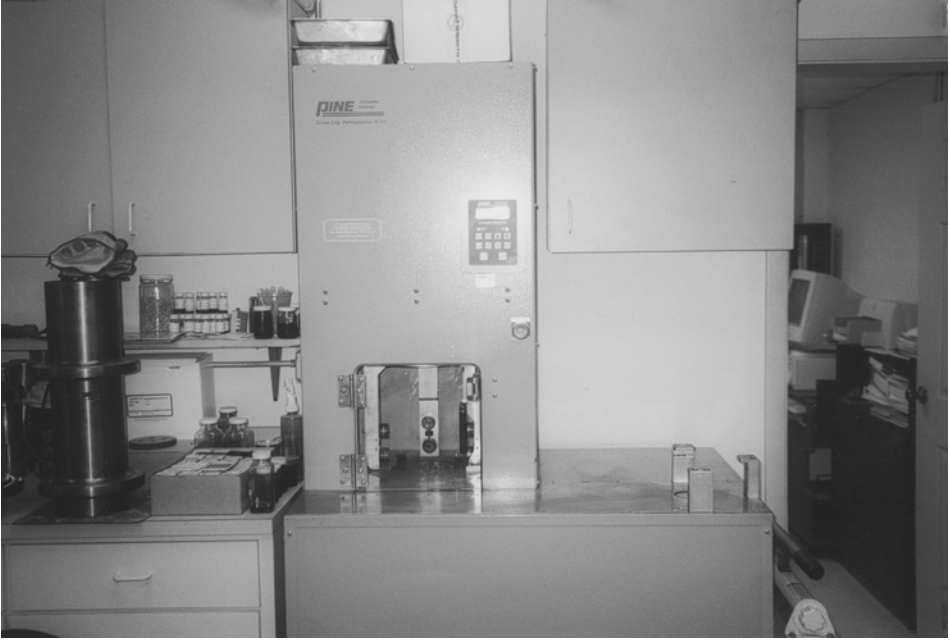
Plate 5.11 SuperPave gyratory compactor.
