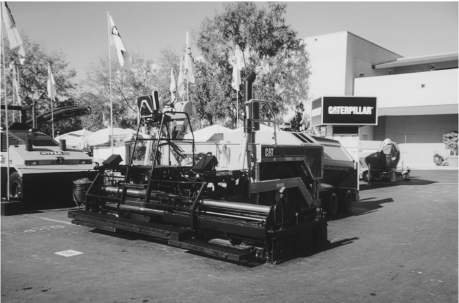
Plate 6.23 Modern asphalt paver.
