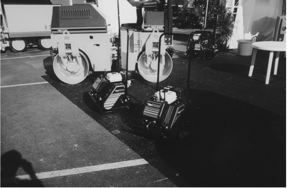
Plate 9.3 Vibrating plate compactors.
