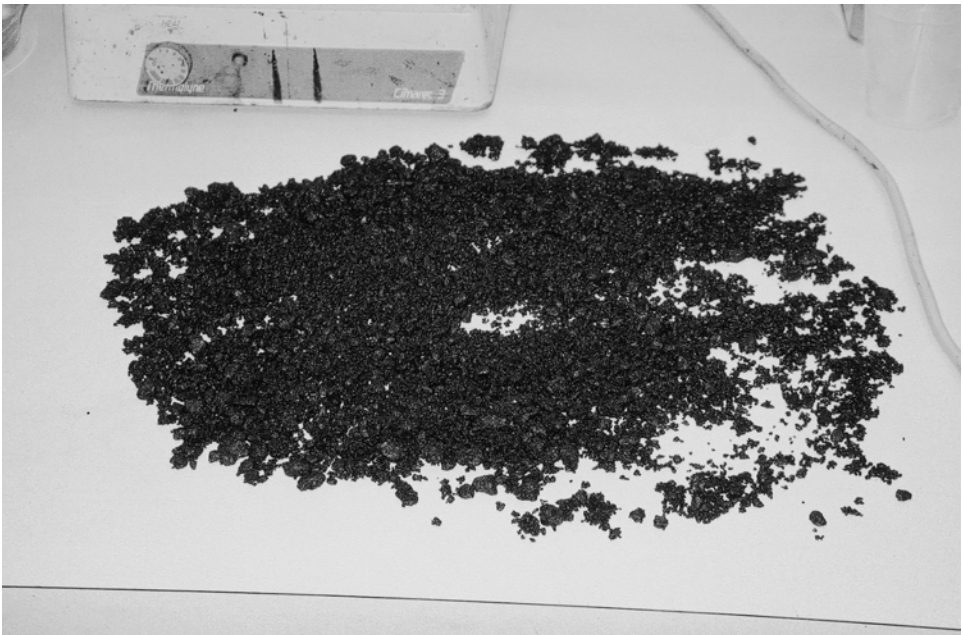
Plate 5.5 Loose mixture for Rice specific gravity.
