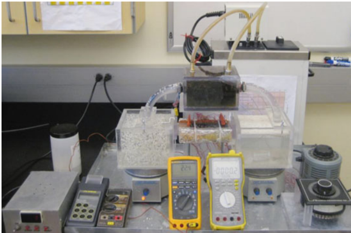
Fig. 21 Final apparatus showing the inlet reservoir ( left ), testing channel ( center ) and outlet reservoir ( right ), with liquid water and microencapsulated phase-change particles, as the bio-inspired multiphase thermal functional fluid, flowing by the exclusive action of the magnetic stirrer placed underneath the inlet reservoir ( left ) [48]
