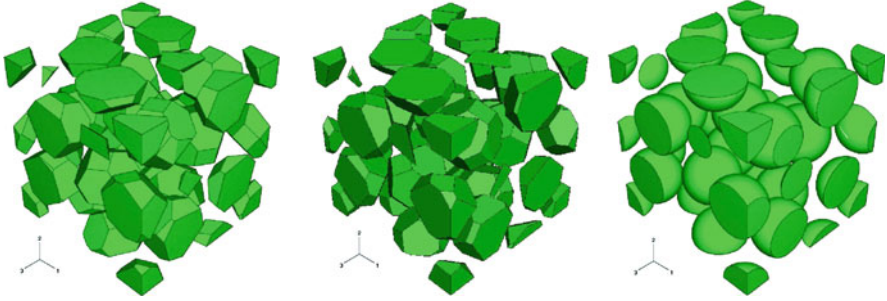
Fig. 8 Three unit cells of nominal particle volume fraction \xi^{(i)} = 0.34 used for modeling the thermal conduction behavior of diamond reinforced aluminum [45]
