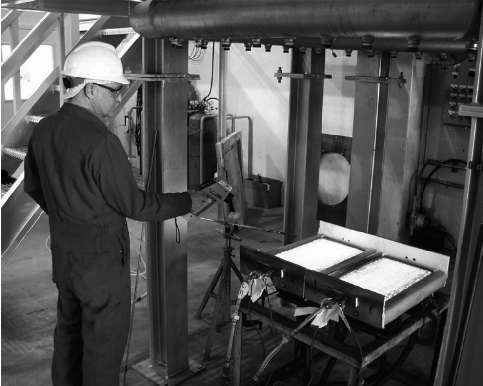
FIGURE 6.9 Example of an infrared pyrometer measuring the surface temperature of a porous refractory matrix burner.
