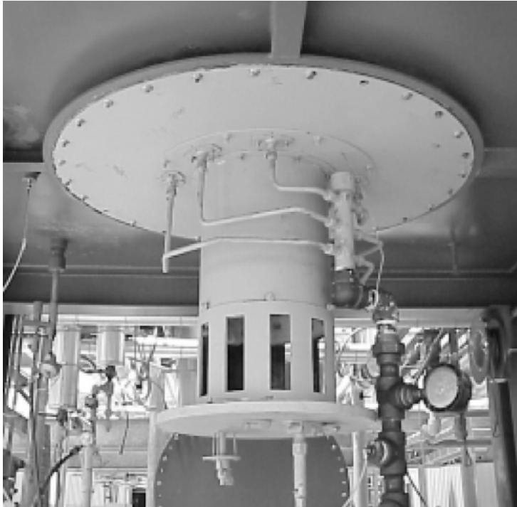
FIGURE 1.19 Natural draft burner. (Courtesy of John Zink Co. LLC, Tulsa, OK. With permission.)
