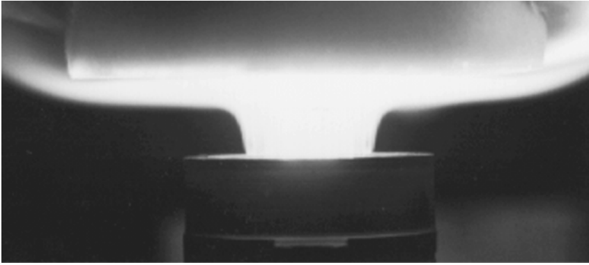
FIGURE 4.7 Natural gas flame impinging on a water-cooled target. (From C.E. Baukal and B. Gebhart, Therm. Fluid Sci. , 15, 323-335, 1997.)
