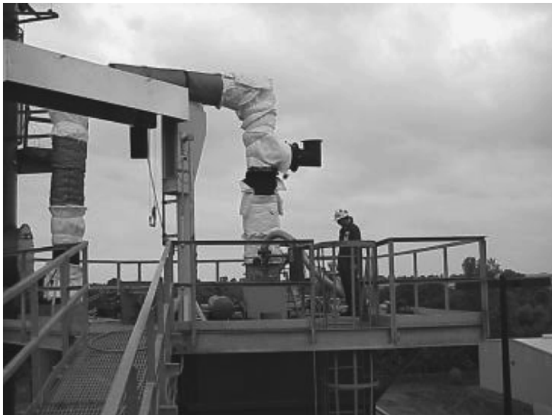
FIGURE 8.45 Example of a down-fired, forced draft, preheated air burner. (Courtesy of John Zink Company, Tulsa, OK.)
