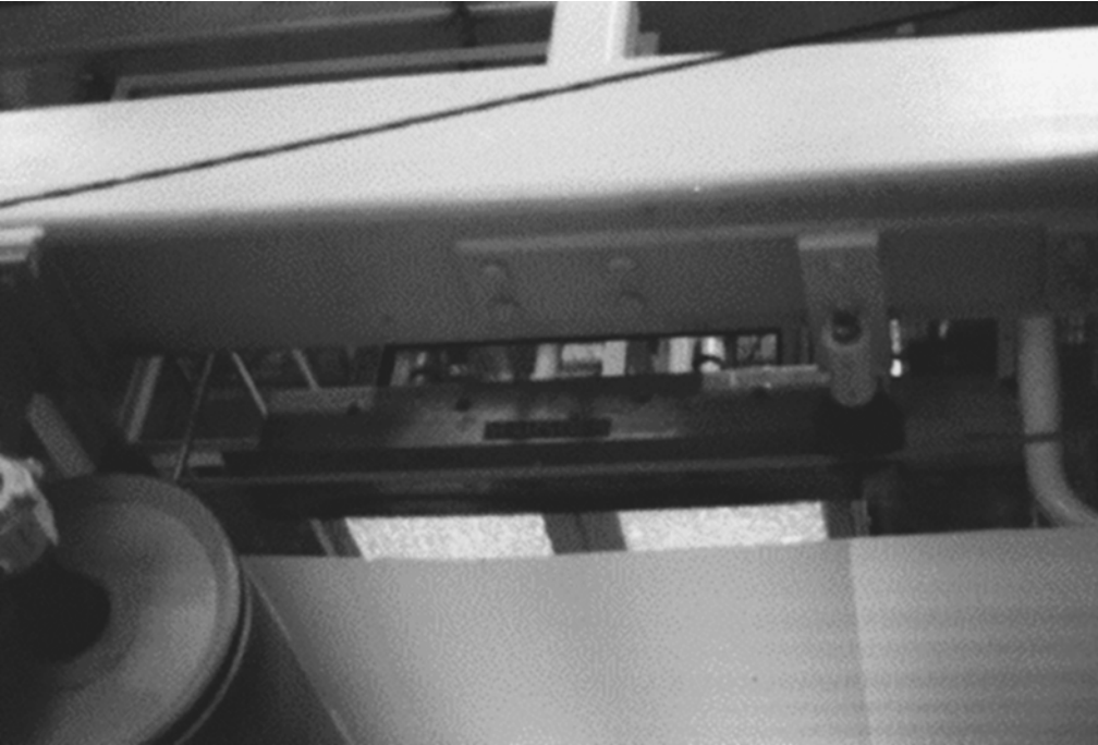
FIGURE 4.4 Infrared burner heating a continuously moving substrate. (Courtesy of Marsden, Inc., Pennsauken, NJ).
