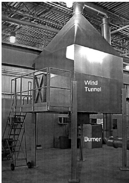
FIGURE 6.12 Wind tunnel simulator for studying fluid flow in a combustor. (Courtesy of John Zink Co. LLC, Tulsa, OK.)
