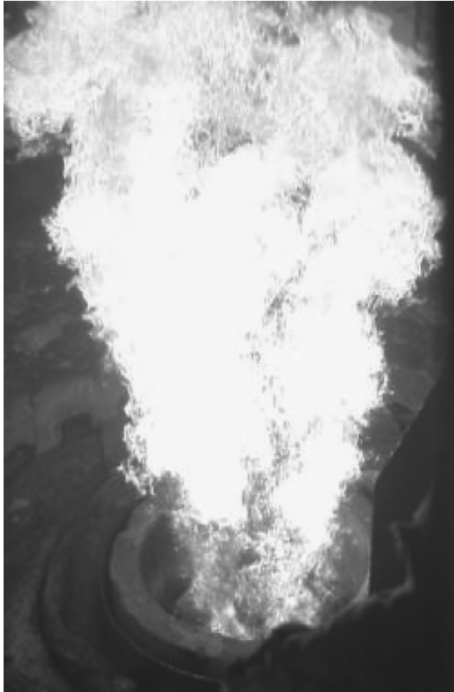
FIGURE 8.2 Example of a high-luminosity oil flame. (Courtesy of John Zink Co. LLC, Tulsa, OK.)
